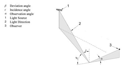
Figure 1. Relevant angles in road lighting design.
