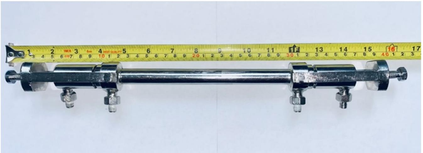
**Figure 5.** Laboratory-scale membrane module with PMP HF.
