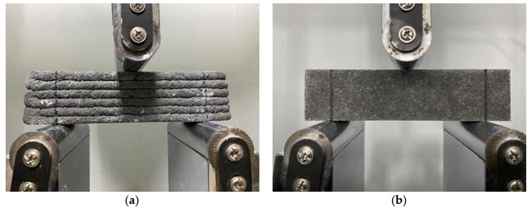
**Figure 6.** The CFRCM flexural test device: (a) 3D printed specimen; (b) cast specimen.
