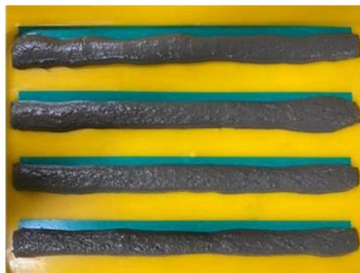
**Figure 3.** Four parallel lines of extruded cementitious mortar.
