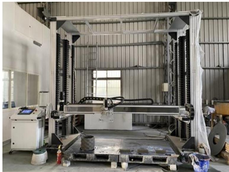
**Figure 4.** The contour craft 3D printer.
