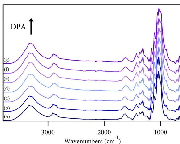
**Figure 1.** FTIR spectra of cotton fibers harvested at different DPA: (a) 18 days post-anthesis (DPA); (b) 20 DPA; (c) 24 DPA; (d) 28 DPA; (e) 32 DPA; (f) 36 DPA; and (g) 40 DPA. Spectra are shown shifted along the y-axis.
