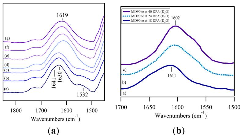
**Figure 3.** (a) FTIR spectra of the O-H bending region for cotton fibers harvested at different DPA: (a) 18 DPA; (b) 20 DPA; (c) 24 DPA; (d) 28 DPA; (e) 32 DPA; (f) 36 DPA; and (g) 40 DPA; (b) O-H bending region (deuterated) harvested at 18 DPA (bottom), 24 DPA (middle), and 40 DPA (top).
