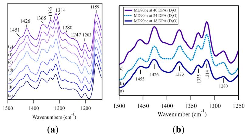
**Figure 5.** (a) FTIR spectra of the fingerprint region for cotton fibers harvested at different DPA: (a) 18 DPA; (b) 20 DPA; (c) 24 DPA; (d) 28 DPA; (e) 32 DPA; (f) 36 DPA; and (g) 40 DPA; (b) Spectra of the fingerprint region of cotton fibers treated with  $\text{D}_2\text{O}$  and harvested at different DPA: (a) 18 DPA (bottom); (b) 24 DPA (middle); and (g) 40 DPA (top).
