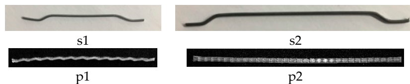
Figure 1. Steel fibers (s1, s2) and macro-synthetic fibers (p1, p2) used in this study.
