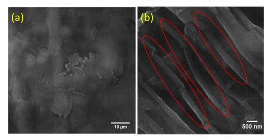
**Figure 2.** SEM images of the GNF before (**a**) and after (**b**) homogenization. (The formation of the GNF is marked in red).
