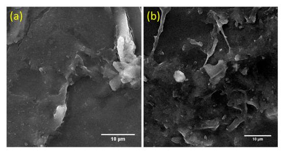
Figure 3. SEM images of the GNF (5%) with Potato starch (a) and Tapioca starch (b).
