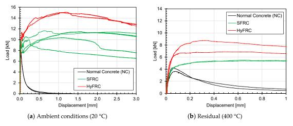
Figure 9. Load-displacement curves obtained from the flexural tests on notched beams.
