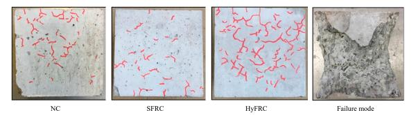
**Figure 3.** Thermal cracks and typical failure mode observed for the cubes used for compressive strength tests after an exposure to maximum temperature of 600 °C.
