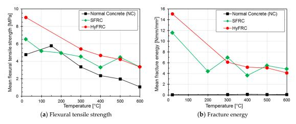
**Figure 10.** Variation of flexural tensile strength and fracture energy as a function of exposure temperature.
