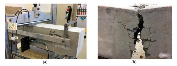
**Figure 8.** (a) Test setup used and (b) close up view of the typical fracture region (failure mode) observed in the flexural tests on notched beams.
