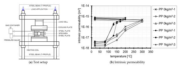
**Figure 2.** Permeability of concrete without and with micro PP fibres as a function of temperature, data from [2]. (Note: 1E-18 refers to  $1.0 \times 10^{-18}$ ).
