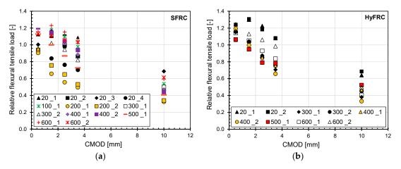
Figure 11. Influence of elevated temperature on the ductility of (a) SFRC and (b) HyFRC.
