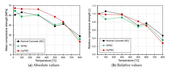
Figure 4. Influence of elevated temperature on compressive strength of different types of concrete.
