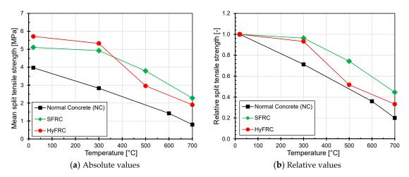
Figure 7. Influence of elevated temperature on split tensile strength of different types of concrete.
