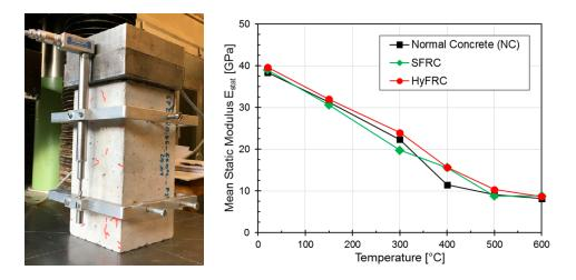
**Figure 12.** (a) Typical test setup and (b) variation of static modulus of elasticity with elevated temperature for different types of concrete.
