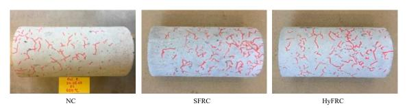
**Figure 5.** Typical thermal cracks observed for the cylinders used for split tensile strength tests after exposure to maximum temperature of 600 °C.
