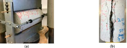
**Figure 6.** (a) Test setup and (b) typical failure mode of concrete cylinders used for determining split tensile strength after exposure to a temperature of 600  $^{\circ}$ C.
