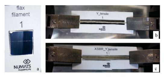
Figure 4. Flax specimens tested in tension: (a) filament; (b) non-impregnated yarn; (c) impregnated yarn.
