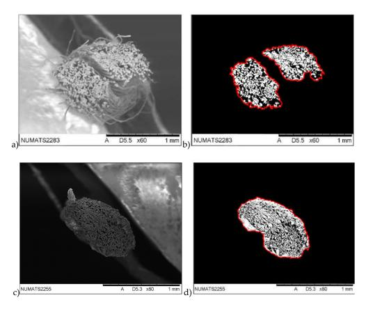
**Figure 3.** Yarns' morphology identification: (a) non-impregnated yarn scanning electron microscope (SEM) image; (b) non-impregnated yarn manipulated SEM image; (c) impregnated yarn SEM image; (d) impregnated yarn manipulated SEM image.
