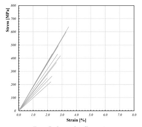
Figure 9. Tensile test results on filament series.
