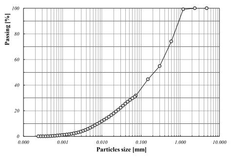
**Figure 1.** Grain size distribution for lime-based matrix.
