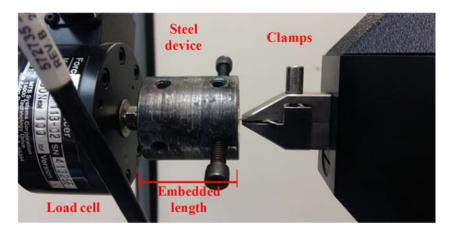
Figure 5. Pull-out test set up.
