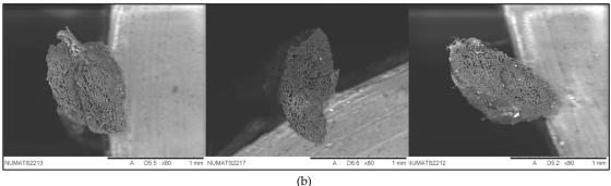
**Figure 6.** SEM images for (a) non-impregnated and (b) Impregnated representative samples subjected to pull-out tests.
