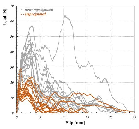
**Figure 11.** Pull-out test results of non-impregnated\_Y\_pull-out and impregnated\_Y\_pull-out series of specimens.
