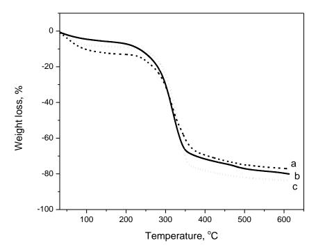
Figure 4. Thermogravimetric (TG) curve of (a) raw CP, (b) CNF procedure I, and (c) CNF procedure II.
