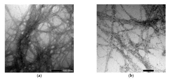
Figure 7. TEM image of (a) CNF procedure I and (b) CNF procedure II.
