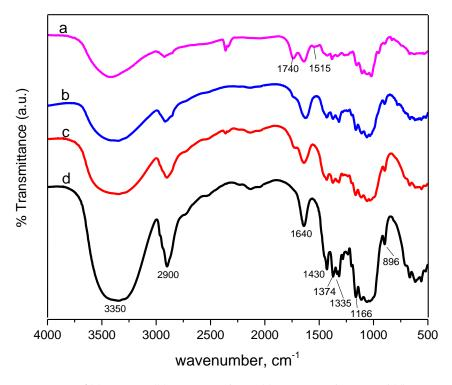
**Figure 2.** FTIR spectra of (**a**) raw CPs, (**b**) CNF procedure I, (**c**) CNF procedure II, and (**d**) microcrystalline cellulose (MCC).
