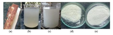
**Figure 1.** (a) Untreated CP, (b) CNF procedure I colloid, (c) CNF procedure II colloid, (d) CNF procedure I powder, and (e) CNF procedure II powder.
