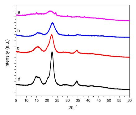
Figure 3. XRD of (a) untreated CP, (b) CNF procedure I, (c) CNF procedure II, and (d) MCC.
