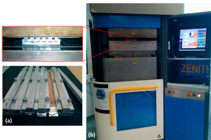
Figure 2. (a) Mold for tensile test samples, and (b) Composite processing in the Pinette hot press.
