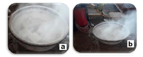
Figure 2. Cooling methods (a) Sudden-cooling; (b) Foam-cooling method.
