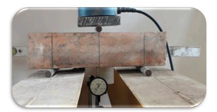
**Figure 11.** A sample of deflection determination for 1.0% V<sub>f</sub> at 400 °C with gradual-cooling method.
