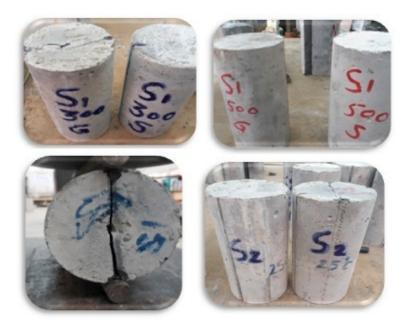
**Figure 7.** RPC samples at different burning temperatures and steel fiber volume fraction percentage after splitting tensile strength test.
