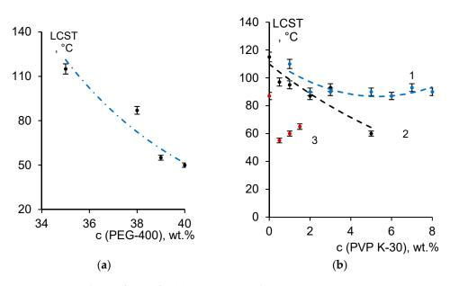
**Figure 2.** Dependence of LCST for (**a**) 20 wt.% PSF solutions in DMA on PEG-400 concentration and (**b**) 20 wt.% PSF solutions in DMA containing, 30 wt.% (1), 35 wt.% (2) and 38 wt.% (3) PEG-400 on PVP K-30 concentration.
