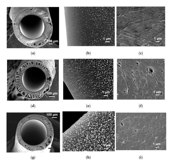
**Figure 4.** SEM micrographs of the membrane cross-section (a,d,g), fragment of the cross-section of the selective layer (b,e,h) and outer surface (c,f,i), obtained from dope solution A (a-c), B (d-f) and C (g-i) at the bore fluid temperature T = 80–83 °C.
