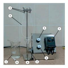
**Figure 1.** Laboratory set-up for the testing of individual hollow fiber membranes: 1—vessel with the feed solution; 2—pump; 3—clamps for fixation of hollow fiber membranes; 4—hollow fiber membrane; 5—manometer (inlet pressure); 6—manometer (outlet pressure); 7—control unit of the pump; 8—measuring cylinder for permeate; 9—pressure regulating valve.
