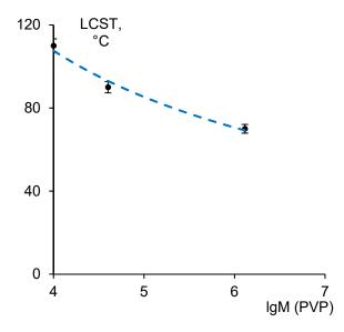
**Figure 3.** The dependence of LCST of the polymer solutions of 20 wt.% PSF 35 wt.% PEG-400, 0.5 wt.% PVP on PVP molecular weight.
