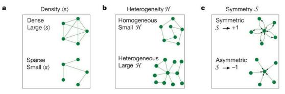
**Figure 2.** Properties determining network behaviour in the event of a failure (taken and modified from [68]).
