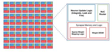
**Figure 8.** Block diagram of the neuromorphic chip proposed by Chen et al. [51]. The architecture consists of 64 neuromorphic cores, connected with a custom NoC. Each core has separate synapse memory and neuron update logic, which can support up to 64 neurons per core. High energy efficiency is achieved with a sparse connection mapping between neurons.
