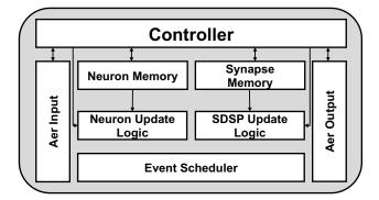
**Figure 6.** ODIN chip block-level diagram by Frenkel et al. [48]. The chip supports a form of online learning based on Spike-driven synaptic plasticity (SDSP). Local neuron memory and synapses memory is used to time-multiplex the dynamics of 256 neurons, using only a single neuron logic. The inputs and outputs of the chip use AER protocol to handle event-driven, asynchronous outputs. The neuron update logic supports both simple LIF and Izhikevich [16] neuron models.
