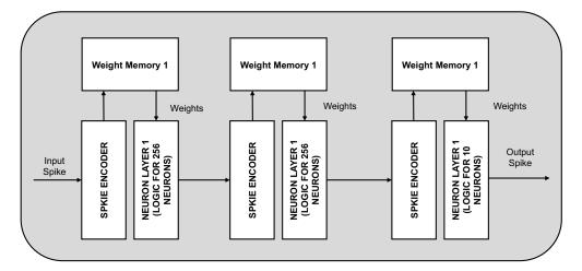
**Figure 7.** Block diagram of the neuromorphic hardware proposed by Yin et al. [49]. The architecture achieves a high level of energy efficiency by fixing the size of the network to a three-layer, 256-256-10 configurations. The input spikes for each layer are encoded by the spike encoder to select only the active neurons. Based on these indexes, corresponding weight values are fetched and loaded to the neurons calculation logic. Dedicated SRAM to store the weights of each layer is included.
