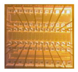
For each ID cell, the value of p was determined by reading from the cell 1000 times, and counting the number of results equal to "1". To find the value of the threshold voltage mismatch,  $\Delta V_T$  in the ID cell, the gate of M1 was held fixed, and the gate of M2 was swept in 1 mV increments. At each increment, the ID cell was read 100 times. From these two measurements, the relationship between p and  $\Delta V_T$  was
