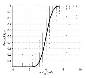
**Figure 6.** Relationship between ID cell error rate,  $\epsilon$ , and the magnitude of the threshold voltage mismatch in the ID cell,  $|\Delta V_T|$ .
