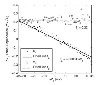
The practical effect of this is that a larger value of  $V_R$  must be selected for reliable operation, due to the combined effects of electronic noise and temperature dependence. For positive values of  $\Delta V_T$ , and if all temperature dependencies are assumed to fall within  $6\sigma$ , then the worst case temperature shift from  $\Delta V_T$  to  $\Delta V'_T$  over an increase in temperature  $\Delta T$  is
