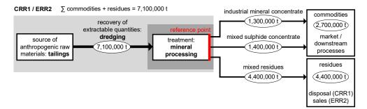
**Figure 4.** Material flow systems and 5-year material flows for the mineral RMs recovery scenarios (CRR1, ERR2). The light grey and dark grey shaded fields illustrate the spatial and mineral processing system boundaries, respectively. All figures were rounded to the sixth digit.
