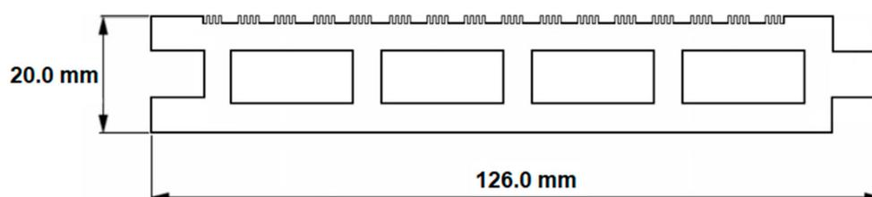
**Figure 1.** Schematic of the hollow-shaped decking board composite profile.
