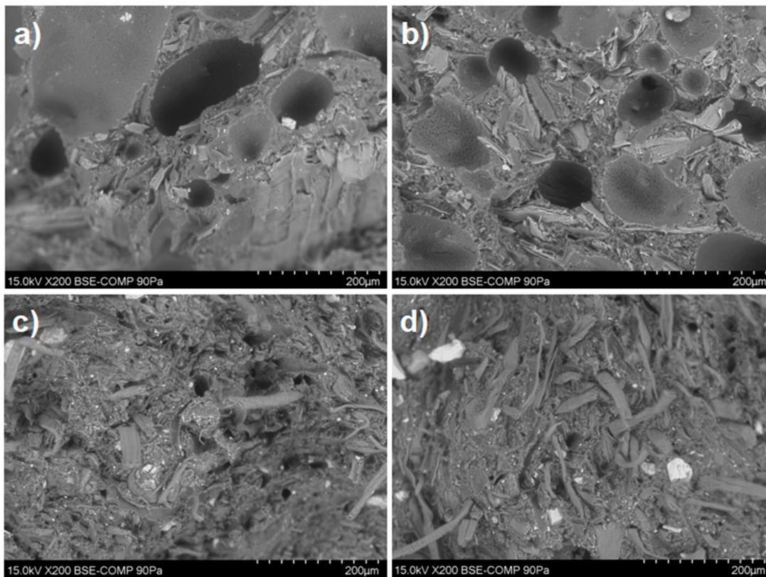
**Figure 4.** SEM images of the cross sections of impact strength samples at a magnification of 200×. Images (a,b) (top) are the before and after images for the reference sample, and images (c,d) (bottom) are the before and after images for the Pr-Sl/HDPE sample. Images (a,c) (left) are before the cyclic treatment, and images (b,d) (right) are the samples after three cycles of the cyclic treatment.
