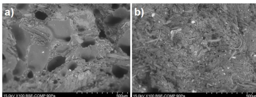
**Figure 2.** Scanning electron microscope (SEM) images of the structure of reference (a) and Pr-SI/HDPE (b) materials, at a magnification of  $\times 100$ .
