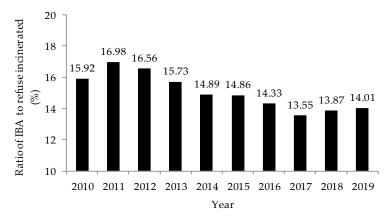
Figure 1. The variations of the ratio of incineration bottom ash (IBA) generation to refuse incinerated since 2010 [12].
