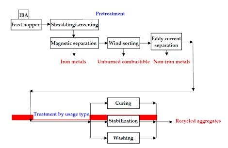
Figure 2. Flowchart of MSW incineration bottom ash (IBA) recycling treatment in Taiwan.
