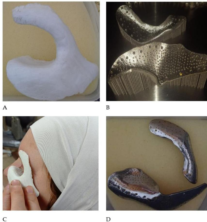
**Figure 5.** Physical printing of the designed PSI parts. (A): plastic prototype, (B): Metallic Titanium PSIs, (C): patient's communication, (D): PSIs after removing the supports, sanding and smoothing.
