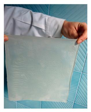
Figure 1. Example of chitin nanofibrils tissue obtained by electrospinning technology.
