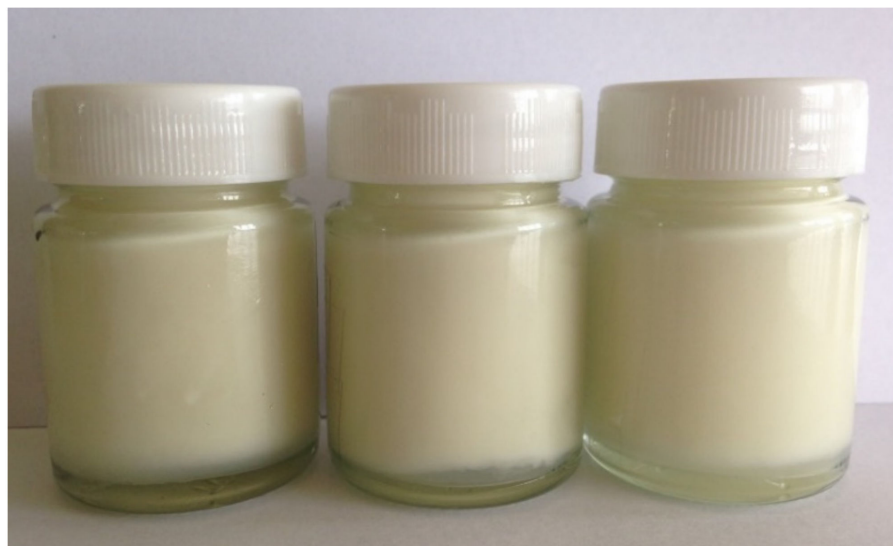
Figure 2. Appearance of the M. oleifera seed oil cream. M. oleifera seed oil cream was prepared by heating stearic acid, stearyl alcohol, cetyl alcohol, and sorbitan ester 80 to 70 °C and incorporating the melted oil phase into the heated water phase (75 °C) containing propylene glycol, polysorbate 80, and deionized water. M. oleifera seed oil (25 g) was gradually added and mixed with the cream base (75 g) under homogenization for 3 min. Concentrated paraben and triethanolamine was added. The pH of the cream base was adjusted using triethanolamine.
