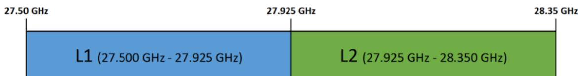
Figure 1. The 28 GHz (27.50–28.35 GHz) local multipoint distribution service (LMDS) spectrum.
