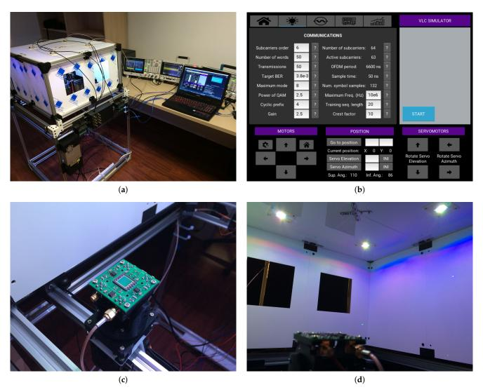
**Figure 12.** Views of the manufactured mockup: (**a**) General view of the experimental testbed. (**b**) Graphical user interface developed in Python. (**c**) Zoom of optical receiver. (**d**) Zoom of emitters at ceiling.
