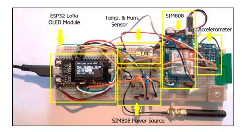
Figure 6. Functional prototype in operation powered with USB Power Bank.
