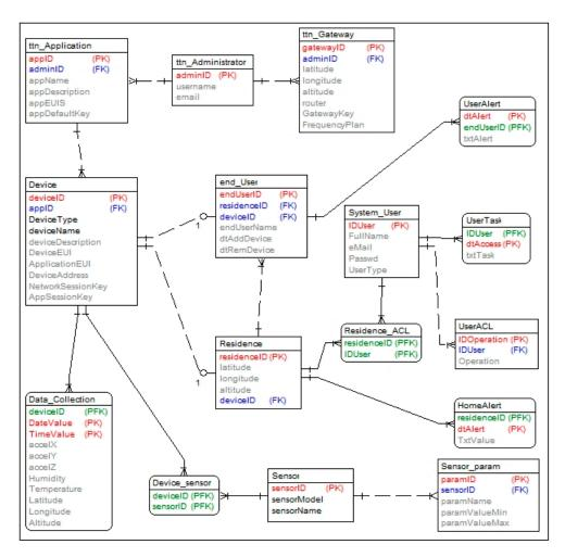
Figure 2. Entity Relational Diagram for IS4HMET.
