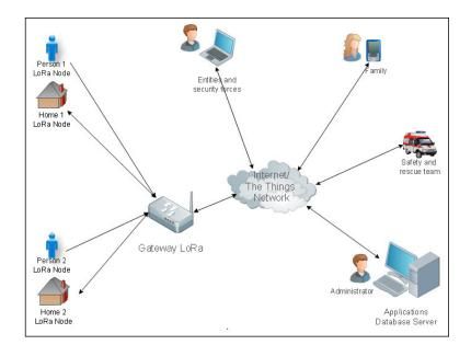
Figure 4. Conceptual scheme of the system.
