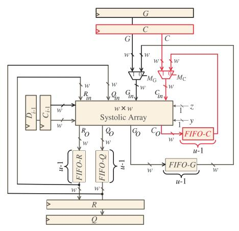
Figure 5. Word-based two-dimensional SISO systolic processor.
