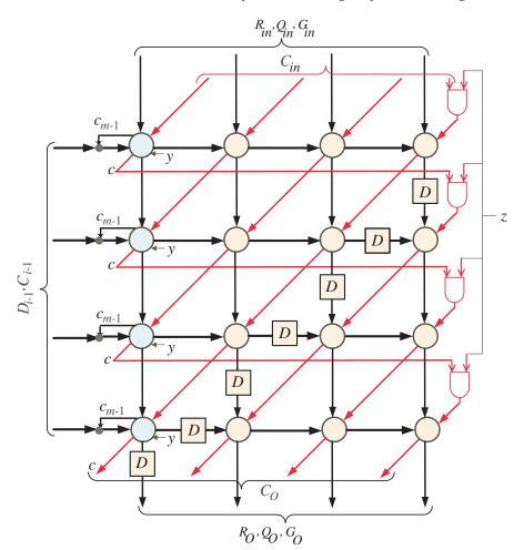
Figure 6. Word-based two-dimensional SISO systolic array.
