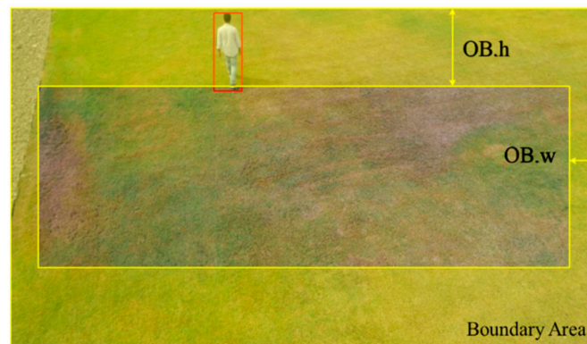
Figure 10. The search range is switching to boundary area when the object is out of bounds.
