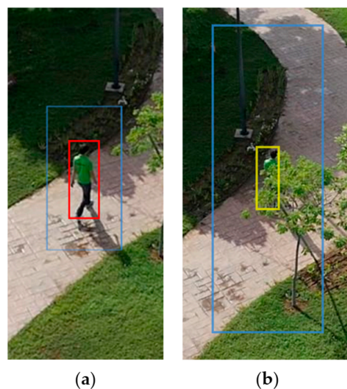
Figure 11. (a) The searching window extends 72 px from the object when unobscured; (b) object occlusion. The yellow box represents the object label of the last mark which was detected successfully; the blue box represents the size of searching windows increases since the PCGF doesn't detect the object.
