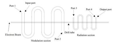
section and radiation section, where the EM wave is cutoff and only electron beam can pass.
