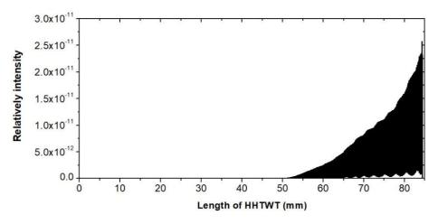
Figure 7. Power curve of the HHTWT at 346 GHz.
