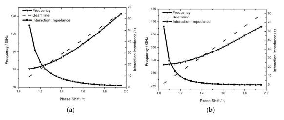
**Figure 2.** High frequency characteristics of the modulation and the radiation section. (**a**) The modulation section; (**b**) the radiation section.
