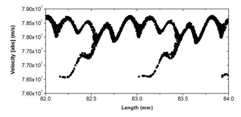
Figure 8. The phase space graph of the electron beam at the end of the radiation section.
