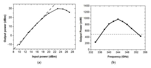
Figure 24. Gain property (a) and bandwidth property (b) of PA-HHTWT.
