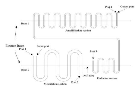
Figure 12. The SWS of the dual-beam CE-HHTWT.
