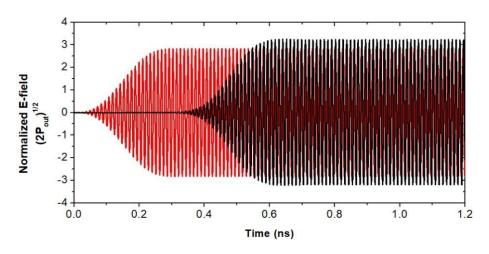
Figure 20. Input (red) and output (black) power of the modulation section at 86.5 GHz.
