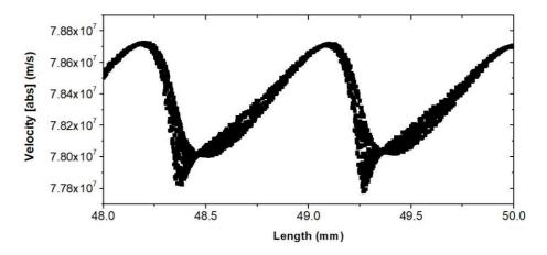
Figure 6. The phase space graph of electron beam at the end of drift tube.
