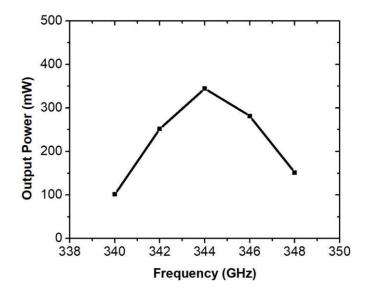
Figure 11. Output power of HHTWT.
