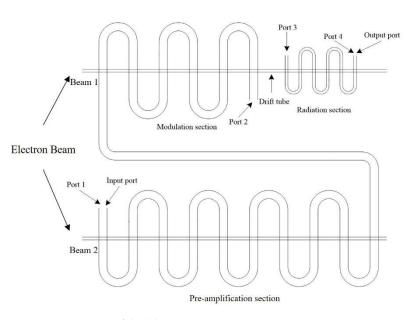
Figure 17. The SWS of dual beam PA-HHTWT.
