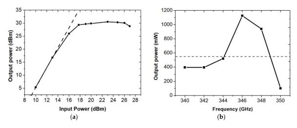
Figure 16. Gain property (a) and bandwidth property (b) of CE-HHTWT.
