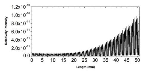
Figure 18. Power curve of the pre-amplification section.
