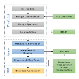
Figure 4. FPGA implementation process.
