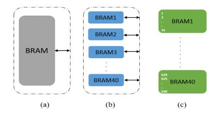
**Figure 5.** Array partitioning: **(a)** without partitioning; **(b)** block partitioning; and **(c)** block with size=16.
