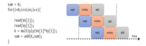
Figure 7. Pipeline directive applied on vector multiplication.
