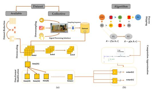
**Figure 1.** Algorithmic level Approximate Computing Techniques: (a) data-oriented; and (b) processing-oriented. Adopted from [17].
