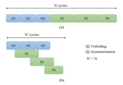
Figure 6. Dataflow pipelining: (a) without dataflow; and (b) with dataflow.
