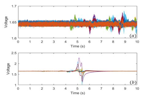
Figure 3. Touch Modalities: (a) touch with noisy readings; and (b) touch with silent intervals.
