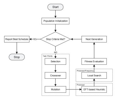
**Figure 2.** The algorithm flowchart of the memetic algorithm (MA)-dynamic voltage frequency scaling (DVFS). EFT, earliest finish time.
