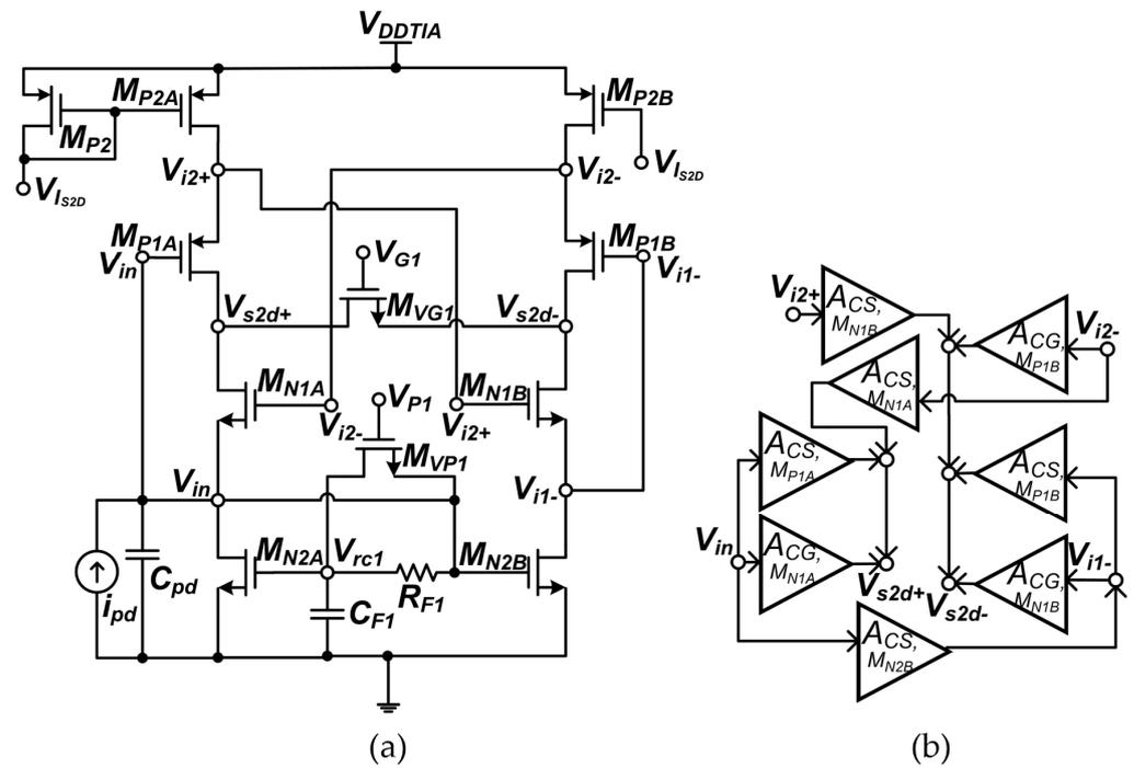
**Figure 2.** (a) Schematic and (b) simplified loop diagram of the proposed TIA single-to-differential input stage.
