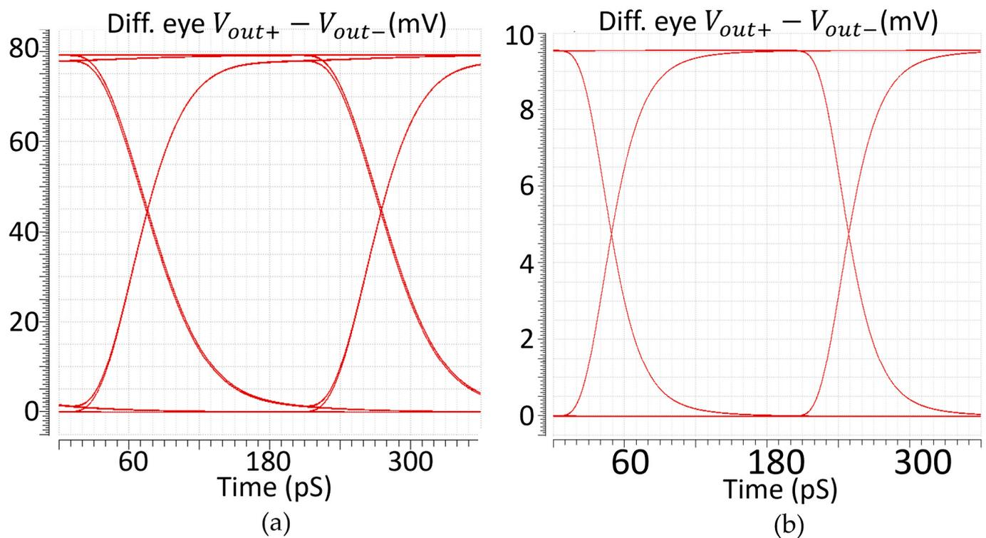
**Figure 10.** Simulated eye diagrams with 5 Gb/s 10 mV<sub>pp</sub> PRBS input signal at (a) maximum and (b) minimum gain settings.
