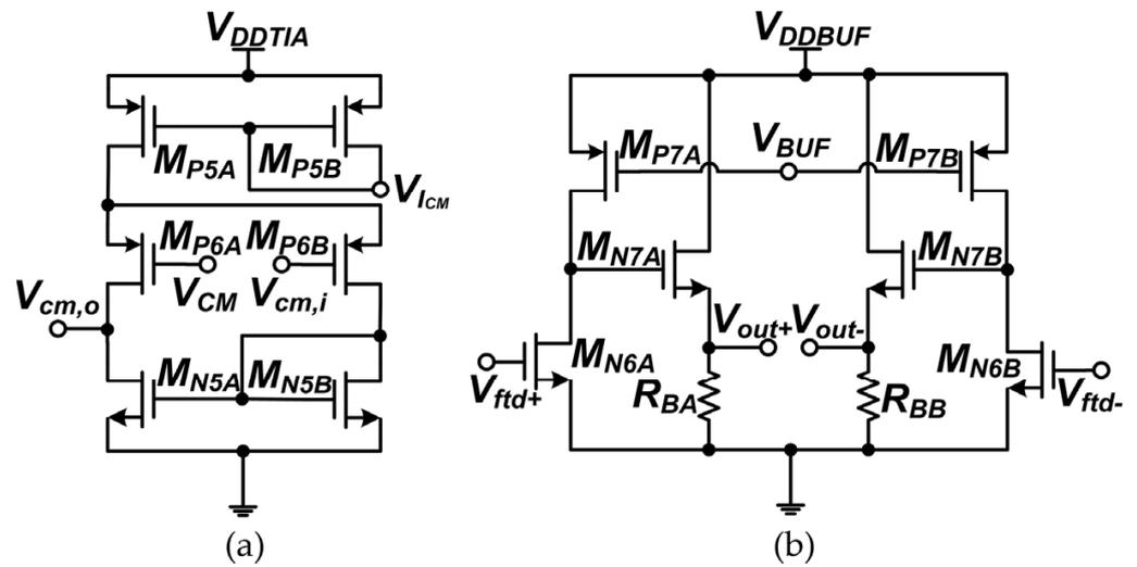
Figure 4. (a) Transistor-level schematic of the CMFB circuit and (b) buffer stage.
