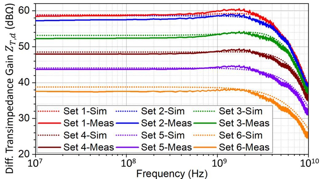
Figure 7. Simulated and measured differential transimpedance gain of the TIA at different gain settings.
