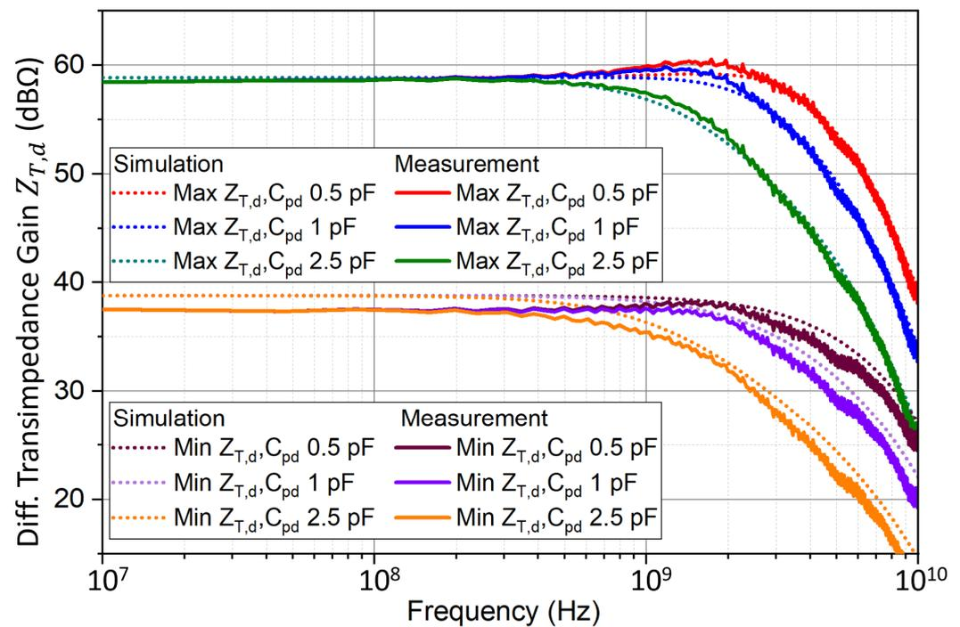
Figure 11. Simulated and measured transimpedance gain of the TIA with range of  $C_{pd}$  values.
