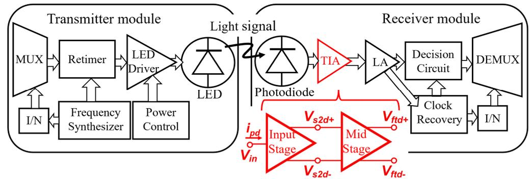
**Figure 1.** Architecture of the transmitter and receiver modules of the VLC system.
