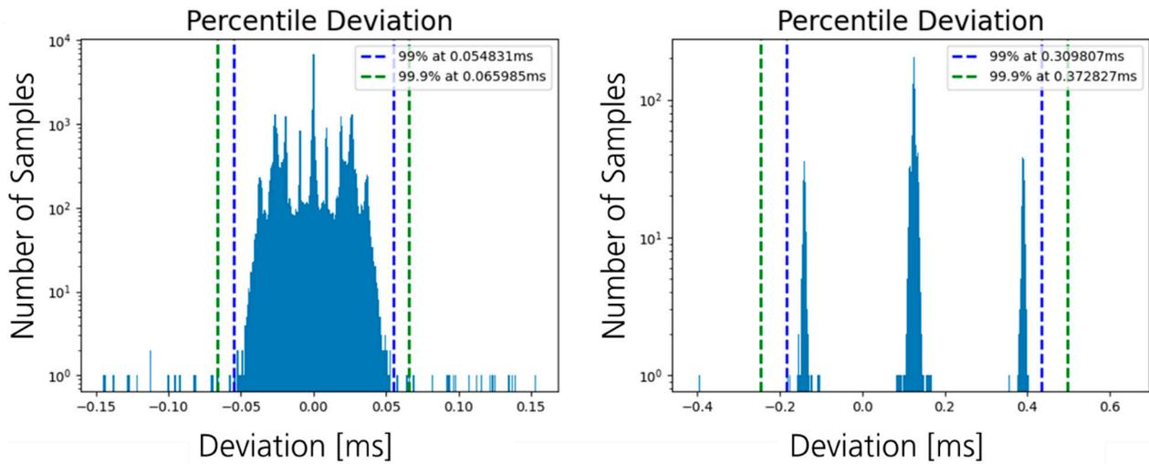
Figure 13. Left: Jitter of the PC output at the network card of the PC. Right: Jitter including over-the-air transmission at the egress gate of TSN-Switch 2 without scheduled traffic.
