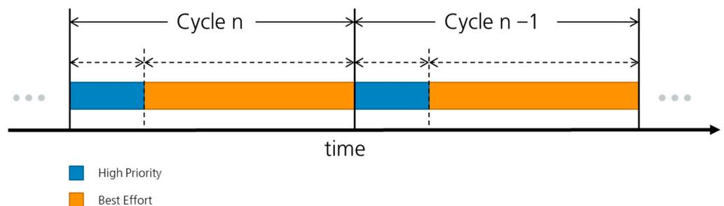
**Figure 3.** Examples of IEEE 802.1Qbv scheduled traffic with two time slots for high priority and best effort traffic.
