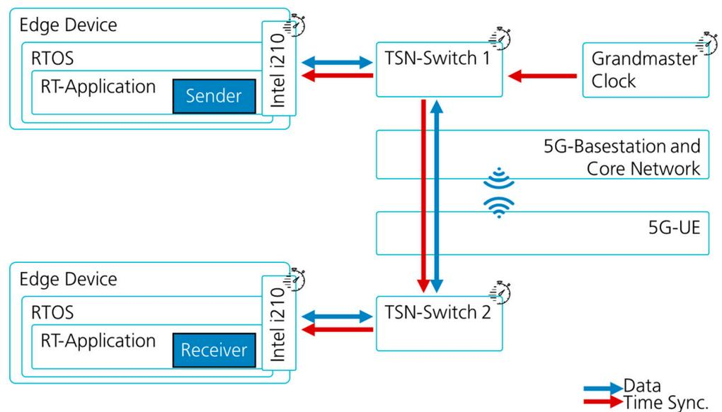
Figure 7. Integration of the 5G-URLLC system in the TSN based network.
