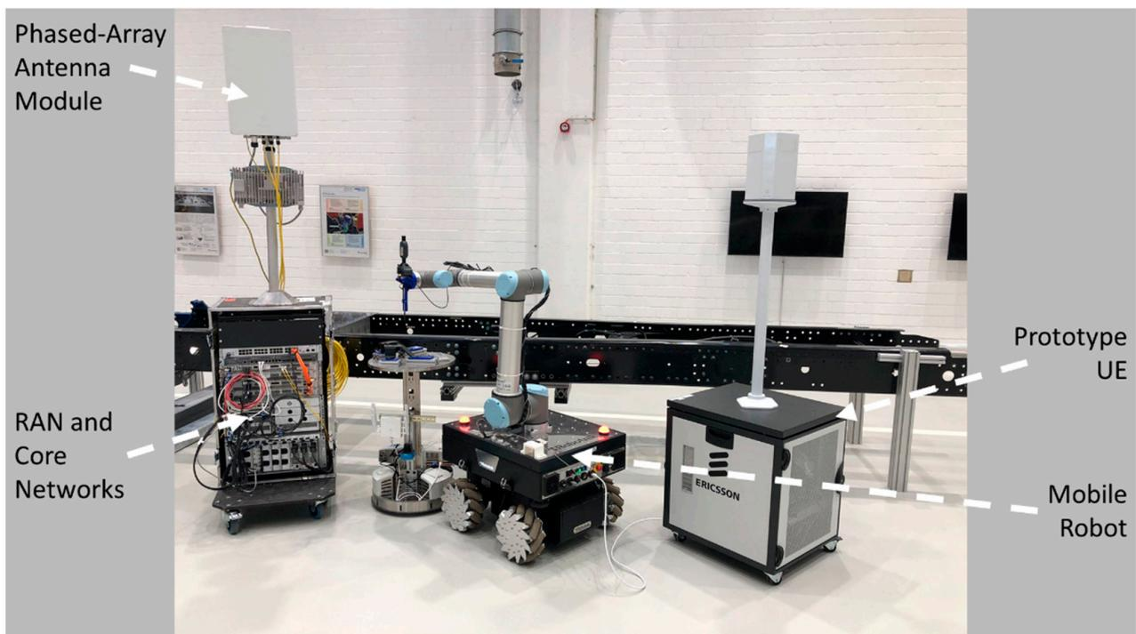
**Figure 4.** Setup of the URLLC testbed and the mobile robot in a shopfloor environment.
