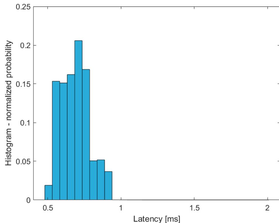
**Figure 5.** Latency histogram of 100,000 samples on the URLLC testbed with UDP traffic with a payload of 32 bytes.
