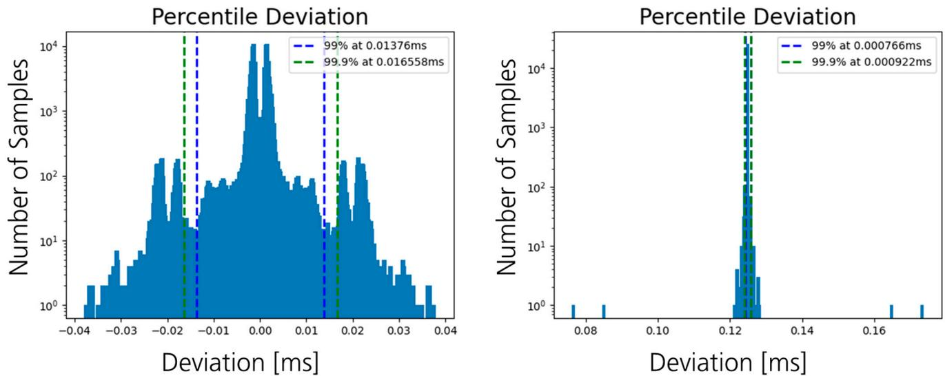
Figure 14. Left: Jitter of the PC output at the network card of the PC. Right: Jitter of the traffic shaped including over-the-air transmissions at the egress gate of TSN-Switch 2 using IEEE 802.1Qbv.
