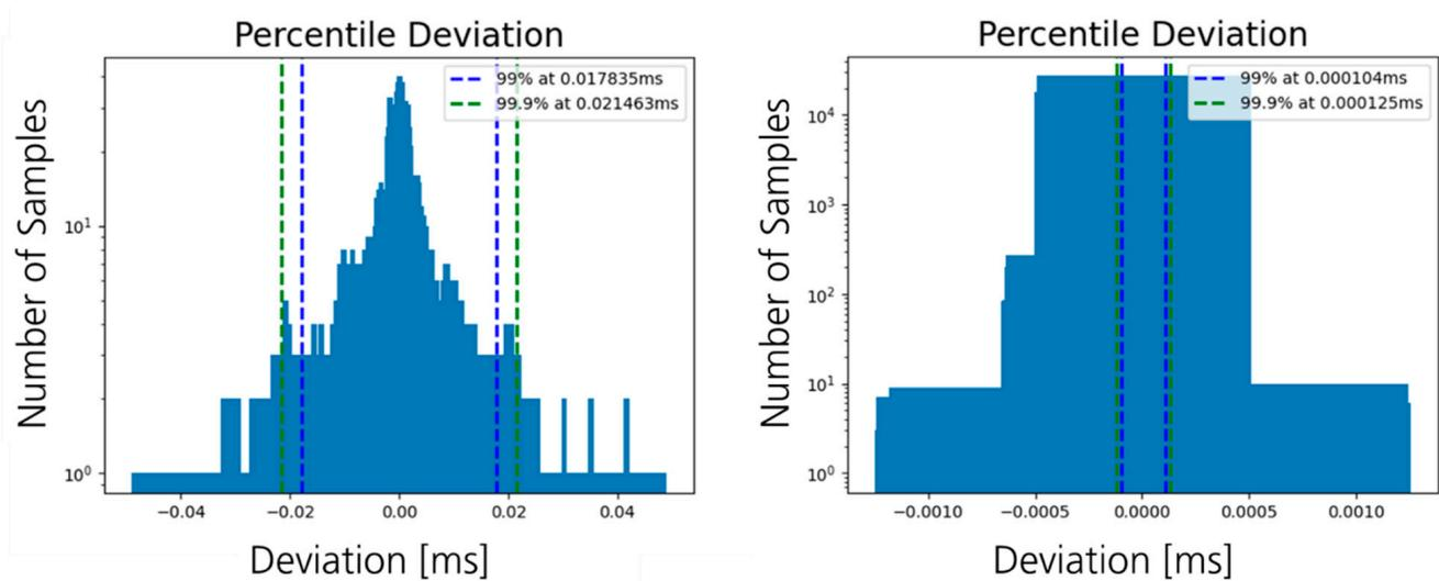
**Figure 12.** Left: Jitter of the PC output at the network card of the PC. Right: Jitter of the shaped PC output at the egress gate of TSN-Switch 1.
