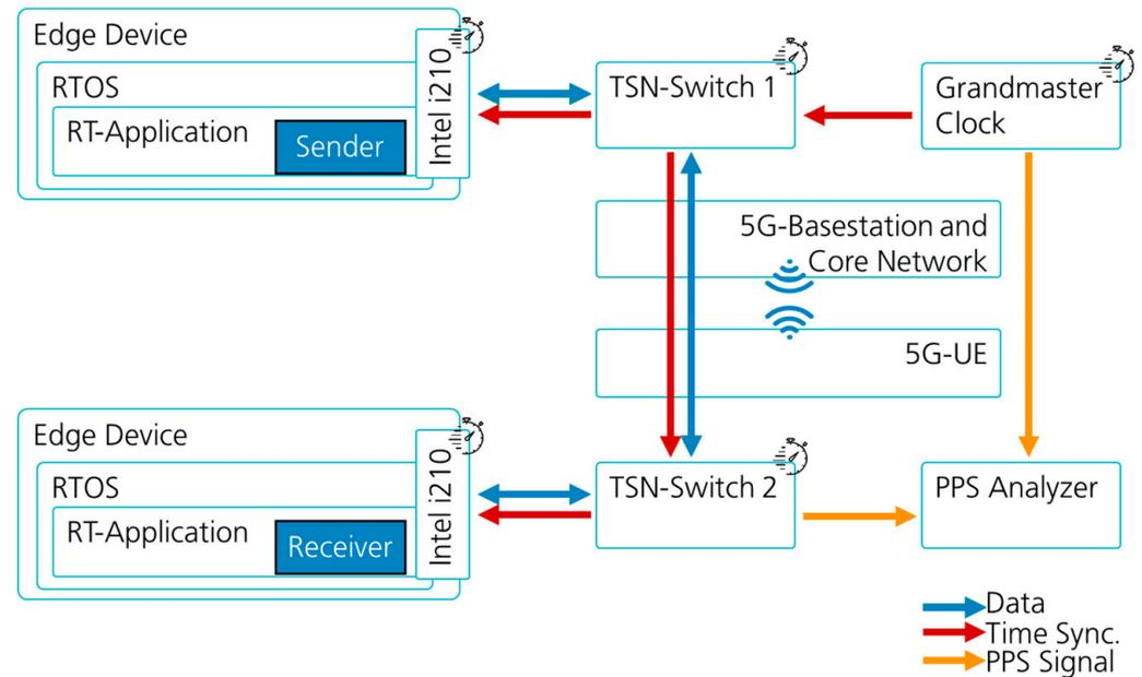
**Figure 8.** Overall Architecture of the Prototype of 5G integrated with TSN.
