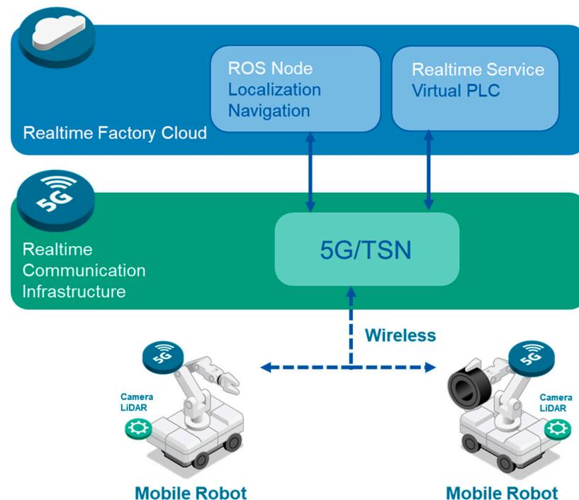
Figure 1. Architecture of a Factory Cloud-Controlled Robotics Application.
