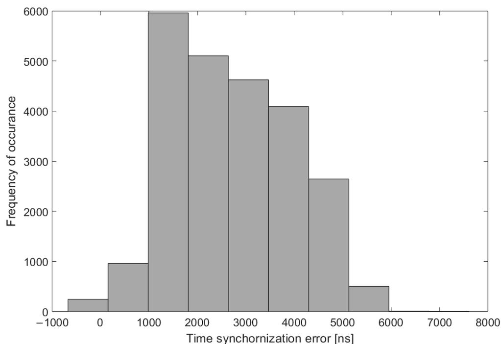
**Figure 11.** Time synchronization error measurements of 5G integrated with TSN.
