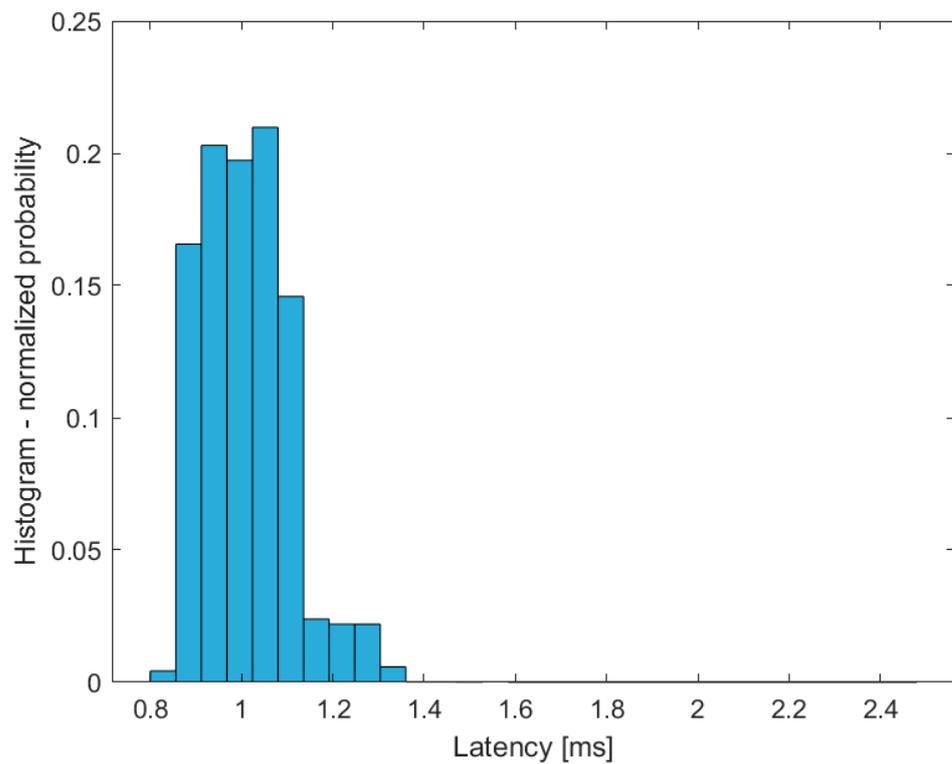
Figure 6. Latency histogram of 100,000 samples on the URLLC testbed with UDP traffic with a payload of 1420 bytes.
