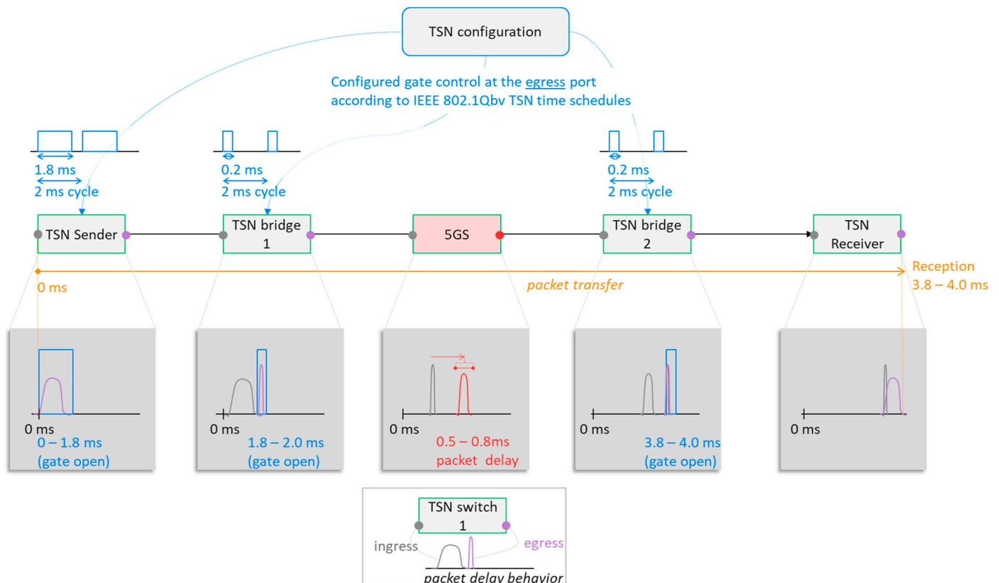
Figure 10. Time shaping carried out in various parts of the setup of 5G integrated with TSN.
