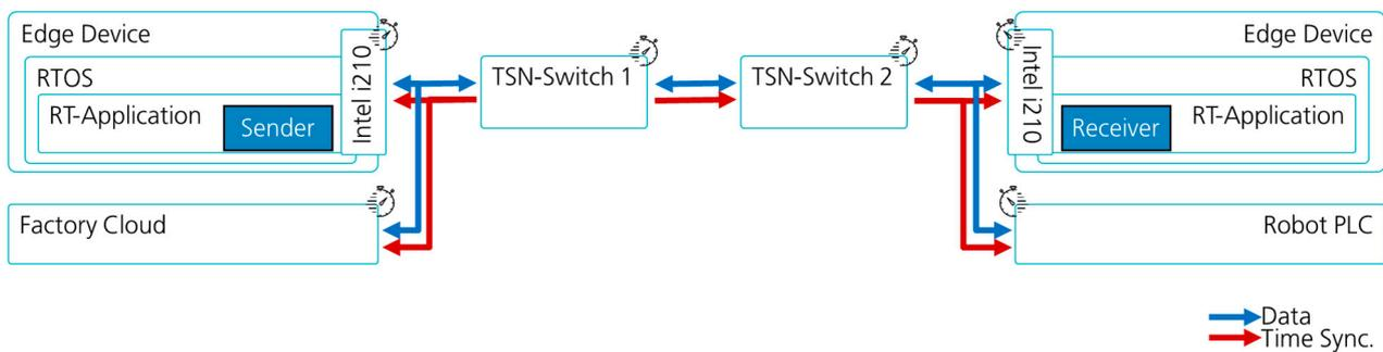
**Figure 2.** Architecture of the TSN setup with connection points for the PLC and the factory cloud.
