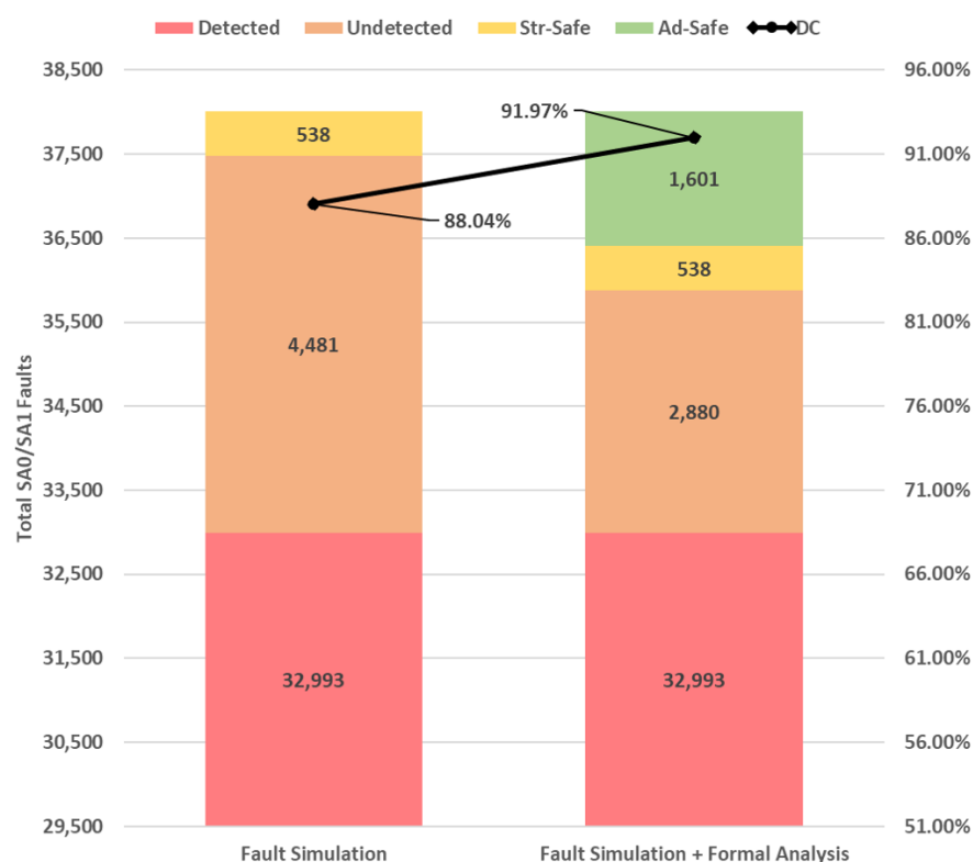
Figure 11. Combined results in CAN: uptrend in DC when fault simulation and formal analysis combined.
