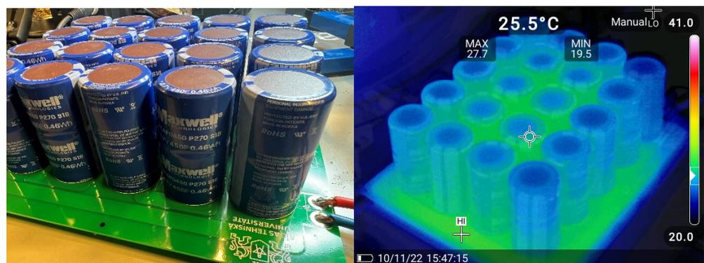
Figure 35. SC energy storage consisting of 20 Maxwell BCAP0450 P270 S18 supercapacitors.
