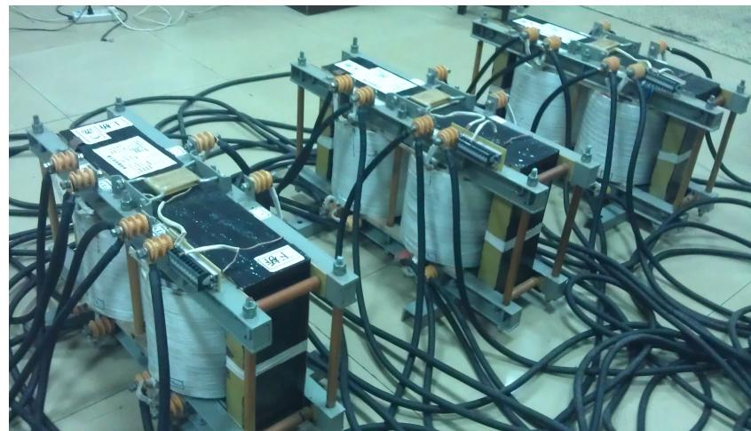
**Figure 3.** Structural model of single-phase transformer.
