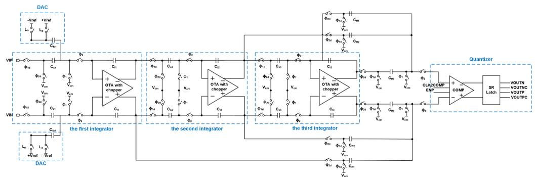
Figure 9. Schematic of the presented third-order modulator.
