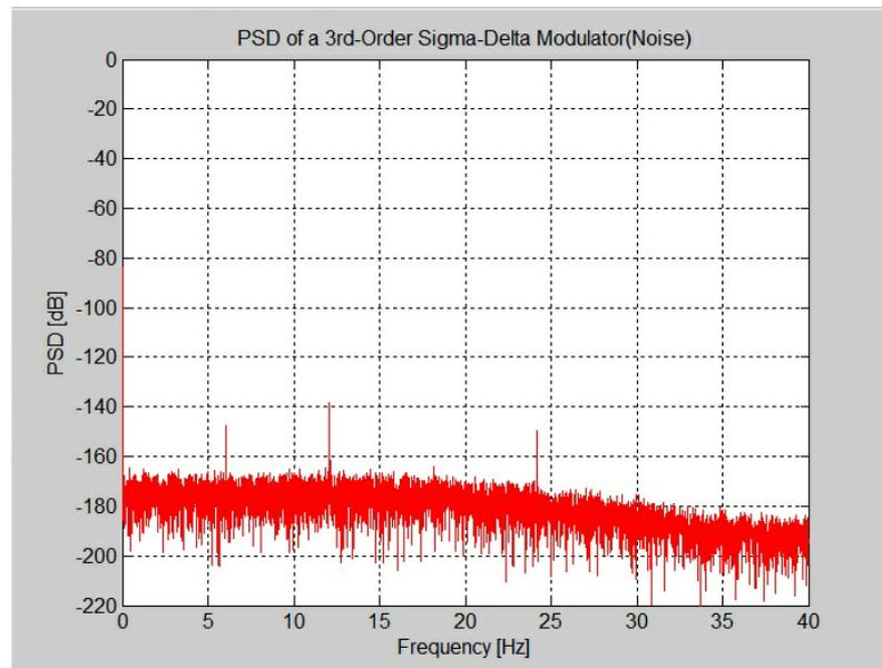
Figure 12. Noise floor of the proposed modulator.
