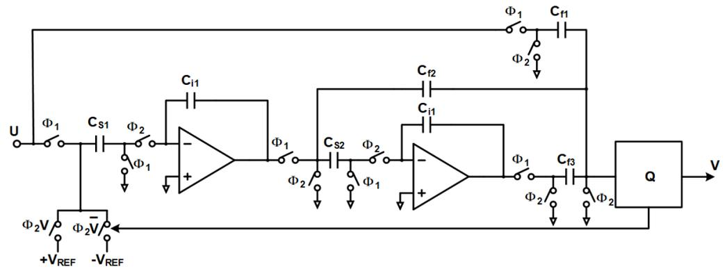
Figure 2. Schematic of the feedforward topology.
