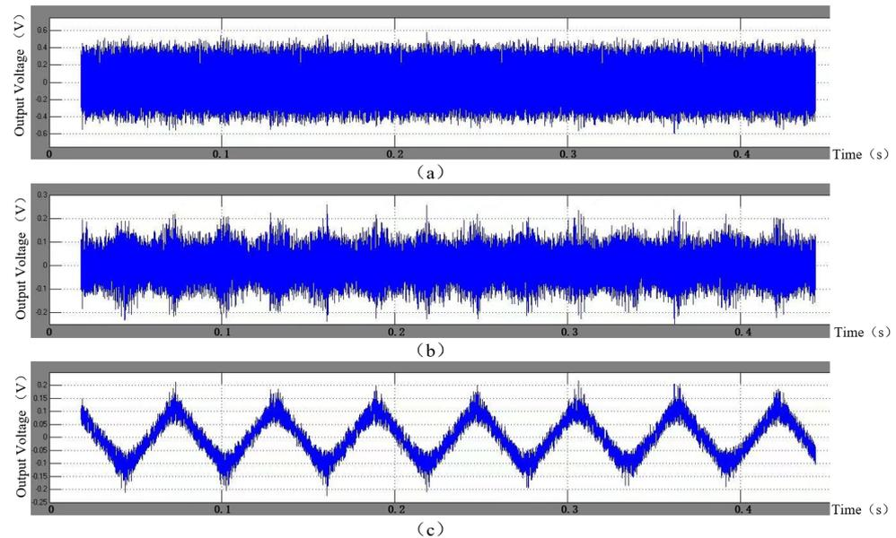
**Figure 5.** Integrator output swings with a 16 Hz full-scale input signal. (a) Output of the first integrator. (b) Output of the second integrator. (c) Output of the third integrator.
