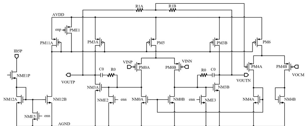
Figure 7. Schematic of the OTA in the modulator.
