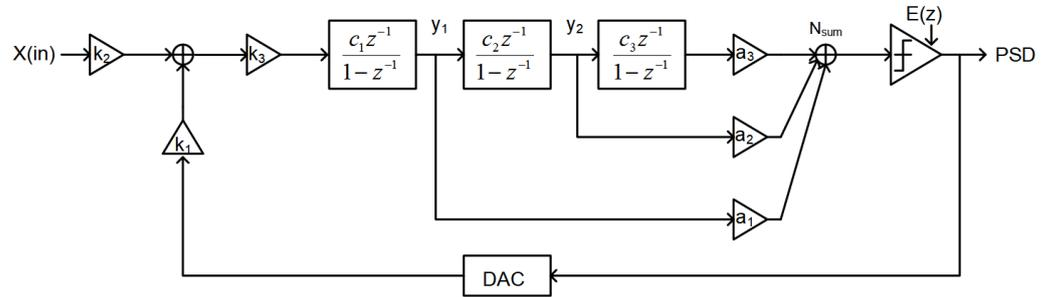
Figure 3. Proposed single-loop third-order modulator topology.
