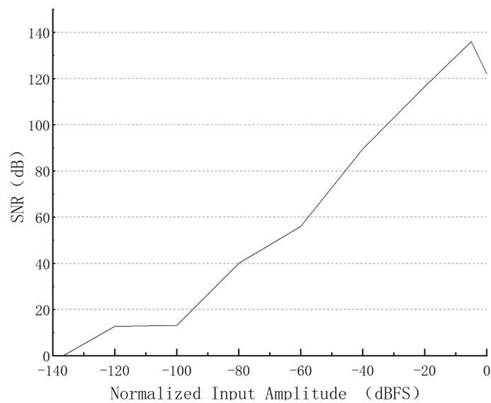
Figure 13. Measured SNR versus the input signal amplitudes normalized by reference voltage.
