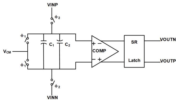
Figure 8. Schematic of the single-bit quantizer.
