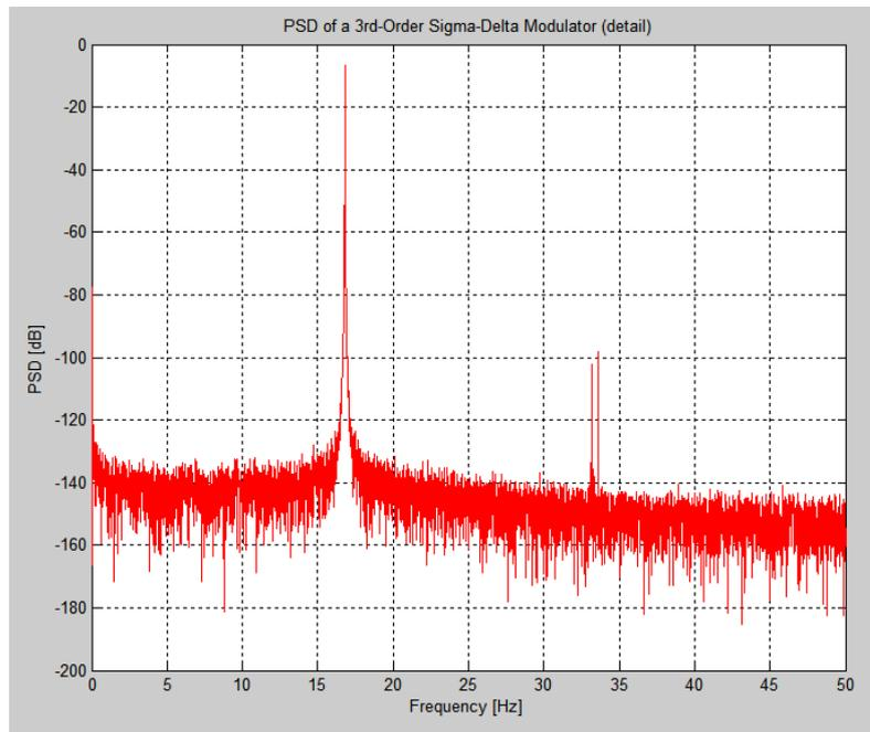
Figure 11. Measured output spectrum with 16 Hz input.
