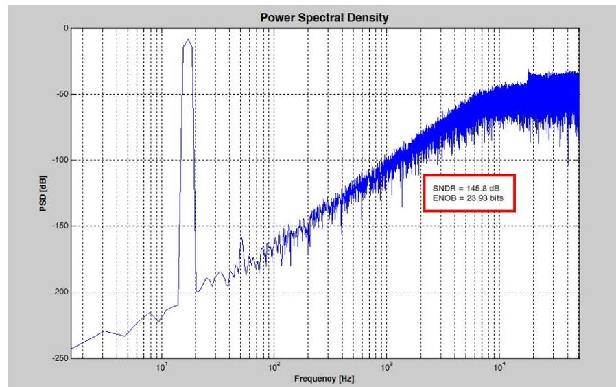
Figure 4. Ideal output spectrum with a 16 Hz input signal.
