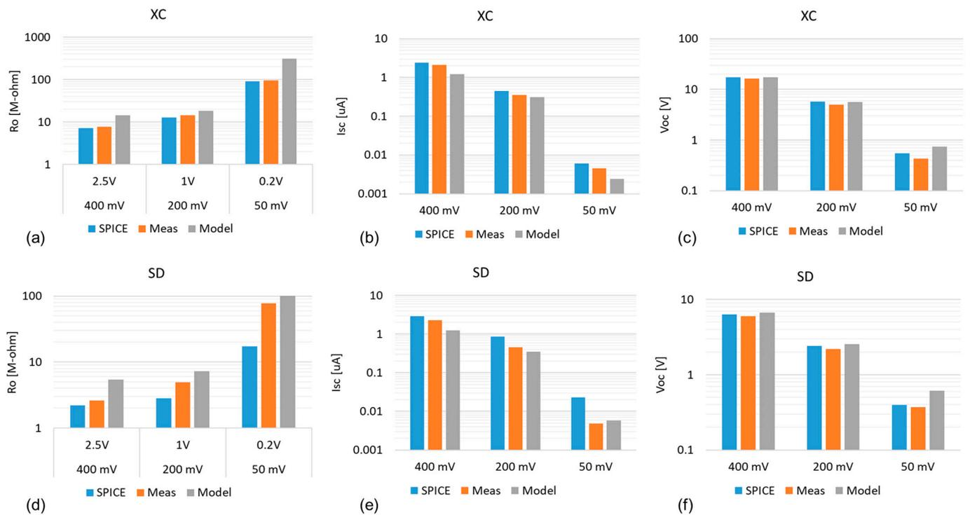
**Figure 18.**  $R_o$  (a),  $I_{sc}$  (b), and  $V_{oc}$  (c) of XC-CP, and  $R_o$  (d),  $I_{sc}$  (e), and  $V_{oc}$  (f) of SD-CP between SPICE, measured and Model (13) results under three conditions of  $(V_{dd}, V_{pp}) = (400 \text{ mV}, 2.5 \text{ V})$ ,  $(200 \text{ mV}, 1.0 \text{ V})$ , and  $(50 \text{ mV}, 0.2 \text{ V})$ .
