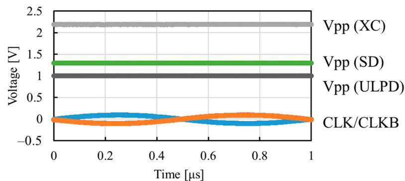
Figure 15. Measured waveform with  $V_{dd}$  of 200 mV and  $f$  of 1 MHz.
