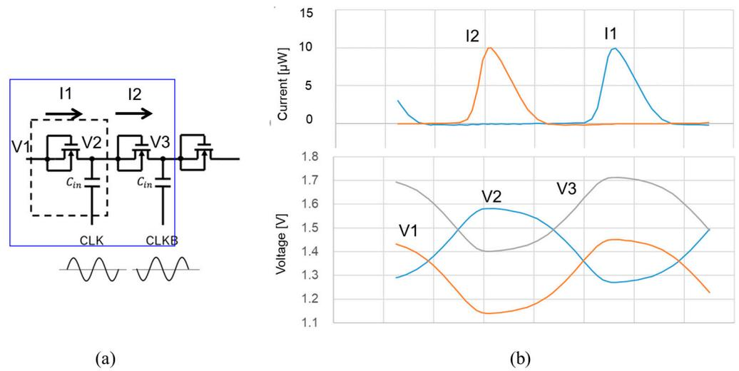
Figure 8. The 12th and 13th stages of SD-CP (a) and their waveforms (b).
