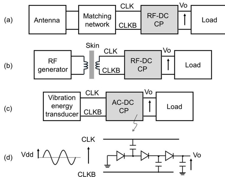
**Figure 1.** Applications of AC–DC/RF–DC CPs (a) Microwave wireless power transmission or RF energy harvesting, (b) biomedical application, (c) vibration energy harvesting) and (d) block diagram of CP.
