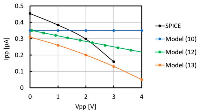
Figure 7. Comparison of  $V_{pp} - I_{pp}$  between SPICE and Models (10), (12), and (13).
