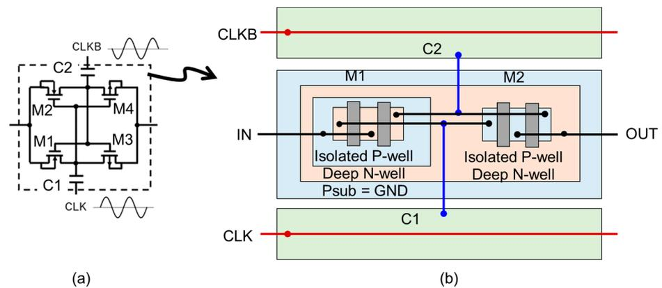
Figure 12. Layout unit of XC-CP (a) and its layout design (b).
