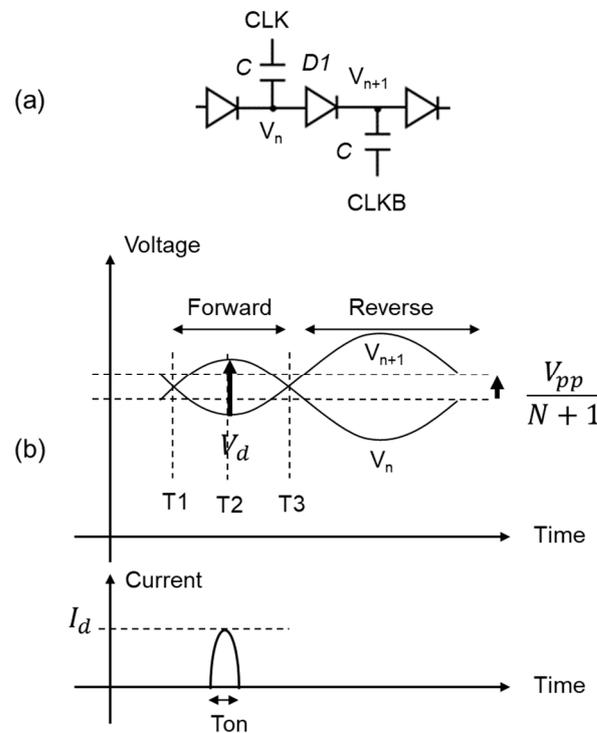
Figure 4. Nodal voltages  $V_n$  and  $V_{n+1}$  of neighboring stages (a) and their waveforms (b).
