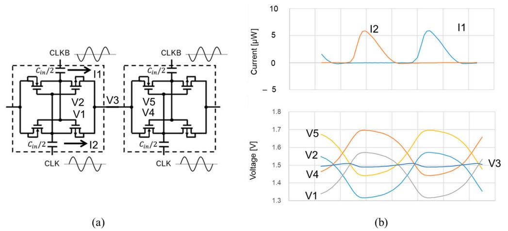
Figure 9. The 12th and 13th stages of XC-CP (a) and their waveforms (b).
