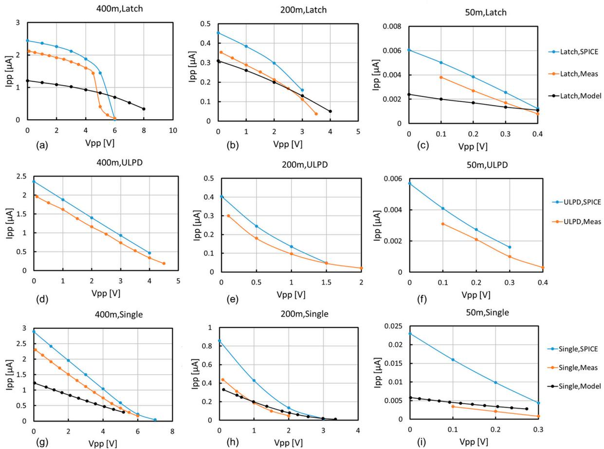
**Figure 17.**  $V_{pp}$ – $I_{pp}$  characteristics: XC–CP (latch) with  $V_{dd}$  values of 400 mV (a), 200 mV (b), and 50 mV (c); ULPD–CP with  $V_{dd}$  values of 400 mV (d), 200 mV (e), and 50 mV (f); SD–CP (Single) with  $V_{dd}$  values of 400 mV (g), 200 mV (h), and 50 mV (i).
