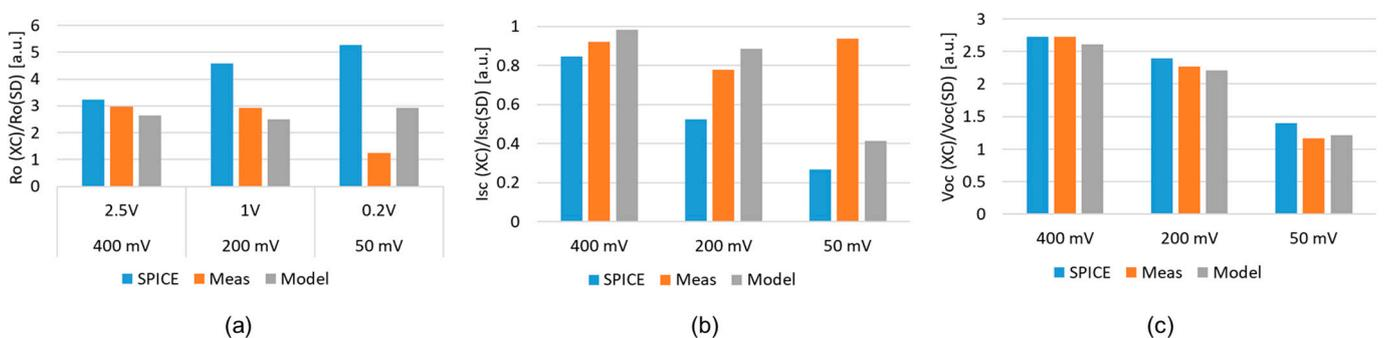
**Figure 19.** Comparison of  $R_o$  (a),  $I_{sc}$  (b), and  $V_{oc}$  (c) of XC-CP normalized by those of SD-CP between SPICE, measured, and model results under the three conditions of  $(V_{dd}, V_{pp}) = (400 \text{ mV}, 2.5 \text{ V})$ ,  $(200 \text{ mV}, 1.0 \text{ V})$ , and  $(50 \text{ mV}, 0.2 \text{ V})$ .
