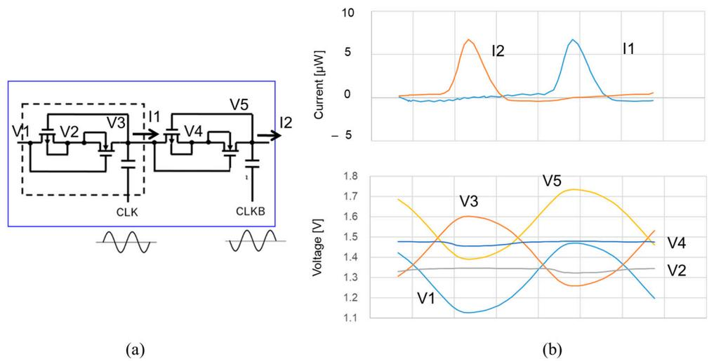
Figure 10. The 12th and 13th stages of ULPD-CP (a) and their waveforms (b).
