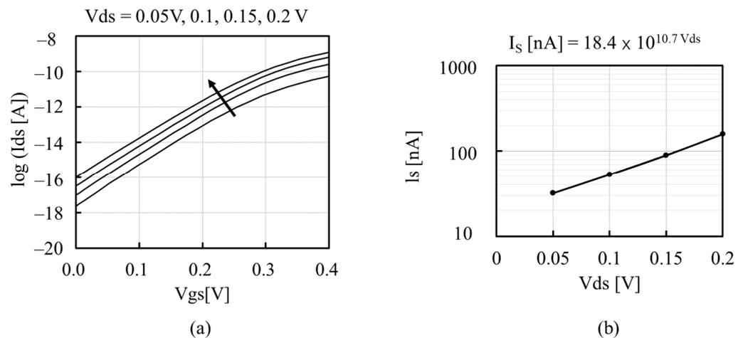
**Figure 6.**  $I_{ds} - V_{gs}$  (a) and extracted  $I_s - V_{ds}$  (b) of an NMOSFET in 250 nm CMOS.
