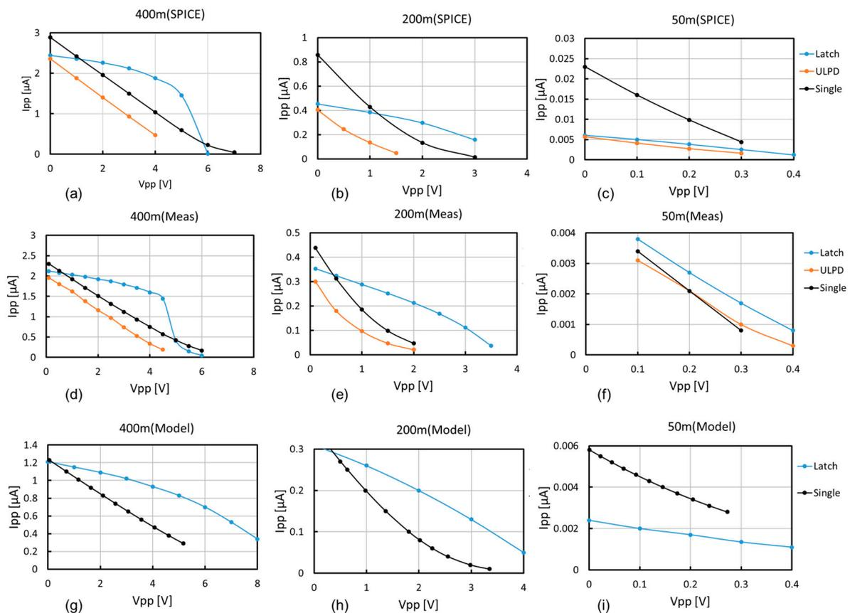
**Figure 16.**  $V_{pp}$ – $I_{pp}$  characteristics: SPICE results with  $V_{dd}$  of 400 mV (a), 200 mV (b), and 50 mV (c); measured results with  $V_{dd}$  of 400 mV (d), 200 mV (e), and 50 mV (f); models with  $V_{dd}$  of 400 mV (g), 200 mV (h), and 50 mV (i).
