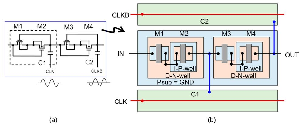
Figure 13. Layout unit of ULPD-CP (a) and its layout design (b).
