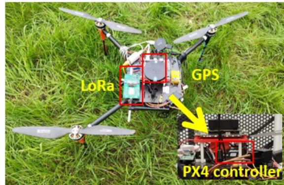
**Figure 2.** The UAV and its hardware layout.
