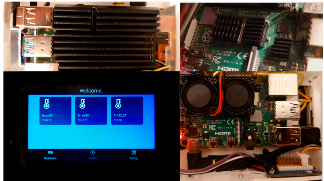
Figure 4. Example of the web interface and cooling methods for a Raspberry Pi [11].
