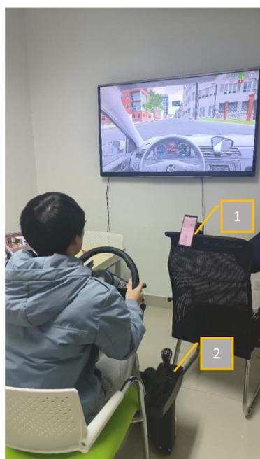
**Figure 9.** Camera location. No. 1 represents the simulated center panel position in the simulation environment; No. 2 represents the simulated rear console position in the simulation environment.
