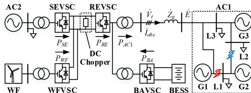
Figure 1. The diagram of the studied three-terminal VSC-HVDC system.
