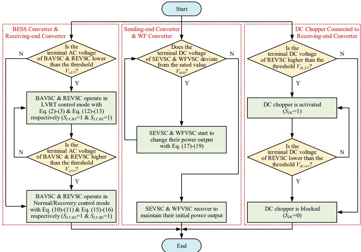
Figure 4. The coordination chart of the equipment under the proposed control strategy during the LVRT and recovery processes.
