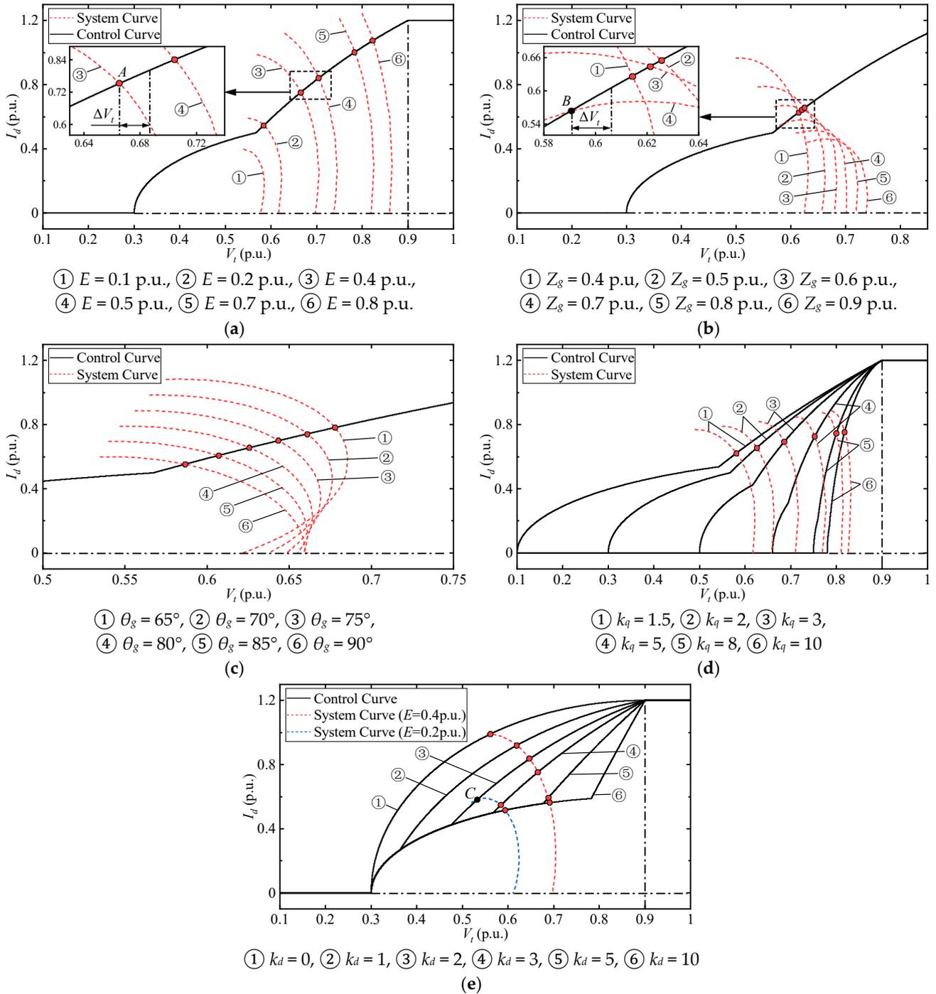
**Figure 5.** The diagrams of the system  $V_t$ - $I_d$  characteristics. (a) when the grid voltage drop  $E$  changes; (b) when the grid impedance amplitude  $Z_g$  changes; (c) when the grid impedance angle  $\theta_g$  changes; (d) when the proportional coefficient  $k_q$  changes; (e) when the proportional coefficient  $k_d$  changes.
