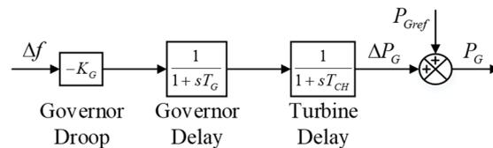
**Figure A1.** The diagram of the generator governor and turbine.
