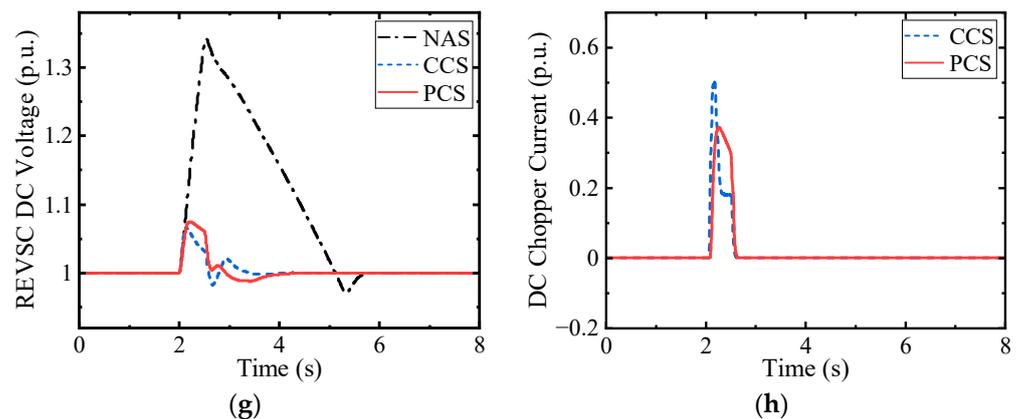
**Figure 6.** The simulation results for deep voltage drop in receiving-end system AC1. (a) The frequency in system AC1; (b) the terminal voltage in system AC1; (c) the active power output of the BESS converter; (d) the reactive power output of the BESS converter; (e) the active power output of the receiving-end converter; (f) the reactive power output of the receiving-end converter; (g) the DC voltage of the DC transmission line; (h) the current in DC chopper.
