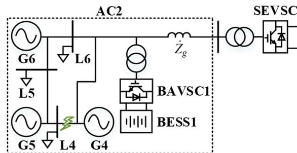
Figure 8. The diagram of the modified sending-end system AC2 with SGs, load nodes, and a BESS.
