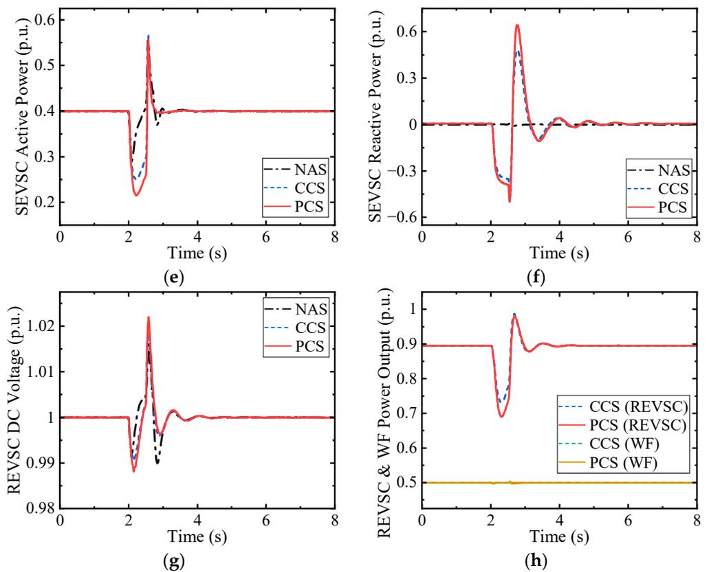
**Figure 9.** The simulation results for deep voltage drop in sending-end system AC2. (a) The frequency in system AC2; (b) the terminal voltage in system AC2; (c) the active power output of the BESS converter; (d) the reactive power output of the BESS converter; (e) the active power output of the sending-end converter; (f) the reactive power output of the sending-end converter; (g) the DC voltage of the DC transmission line; (h) the active power output of the receiving-end converter and WF.
