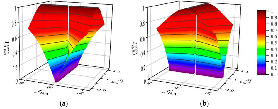
**Figure 3.** The effects of  $f_{BA}$  and  $V_{t,BA}$  on the active and reactive current limitations. (a) The effect of  $f_{BA}$  and  $V_{t,BA}$  on active current limitation; (b) the effect of  $f_{BA}$  and  $V_{t,BA}$  on reactive current limitation.
