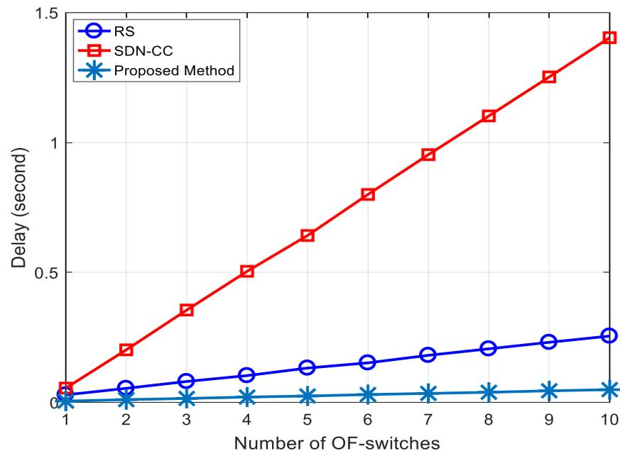
Figure 10. The delay in terms of the number of OF-switches.
