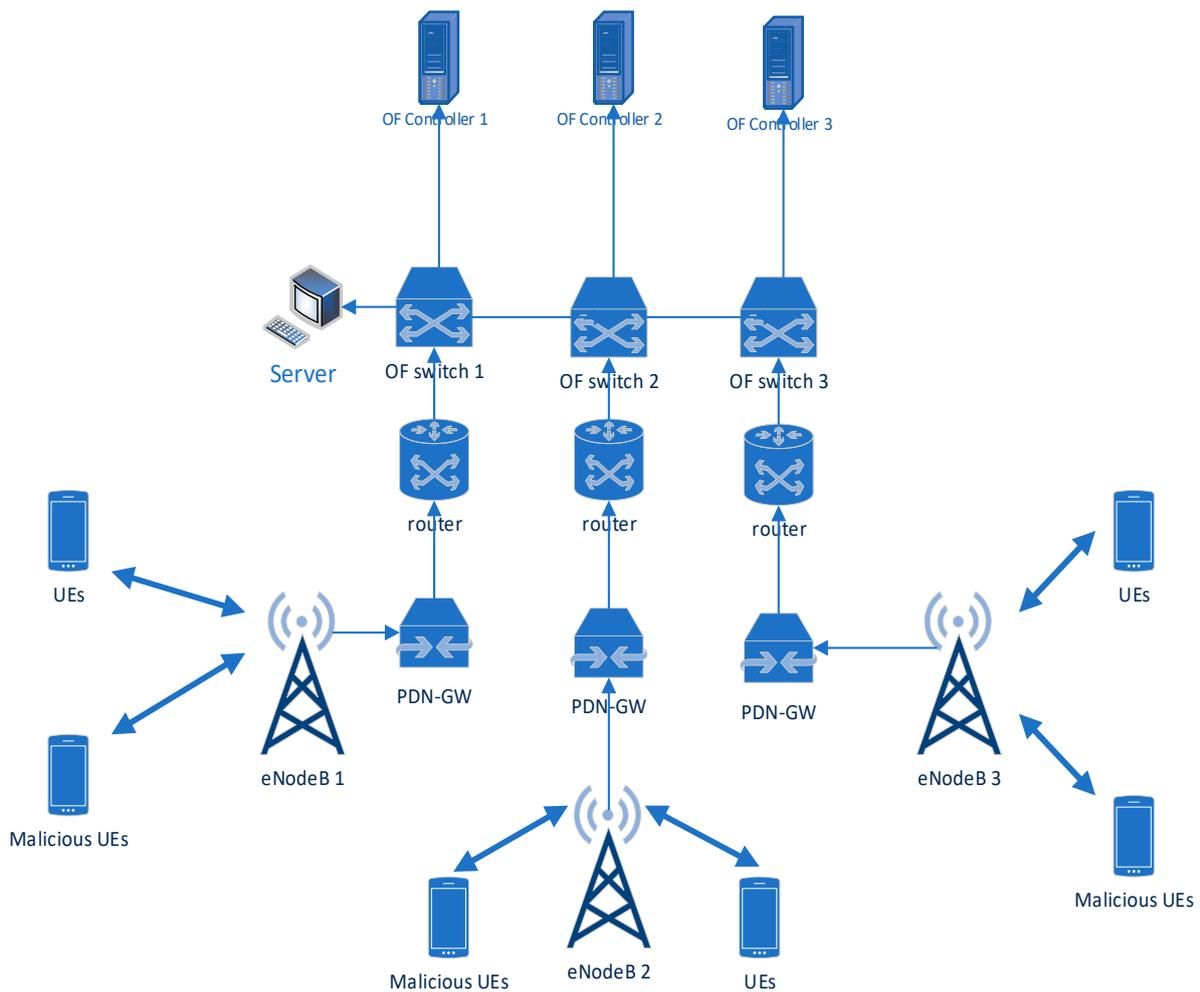
**Figure 3.** The proposed multi-controller (3 controllers) SDN management architecture.
