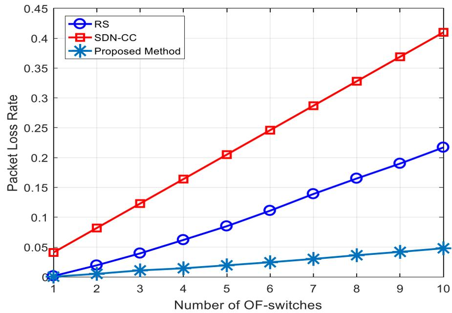
Figure 8. The packet loss in terms of the number of OF-switches.
