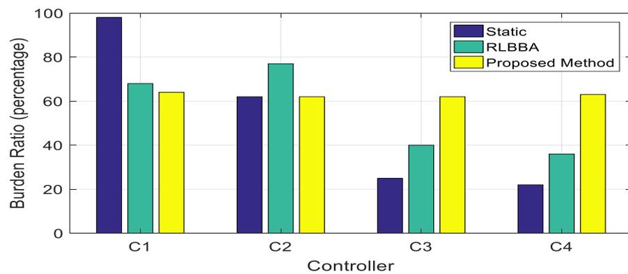
**Figure 5.** Burden ratio of distributed controllers for various burden balancing approaches.
