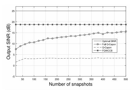
**Figure 9.** Output SINR versus snapshot number with SNR = SIR = 15 dB and  $5^{\circ}$  error.
