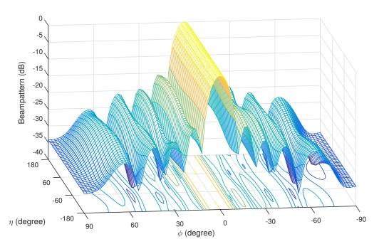
**Figure 5.** The resultant full quaternion worst-case constraint beamformer (FQWCCB) beam pattern with  $\theta = 90^{\circ}$  and  $\gamma = 60^{\circ}$ .
