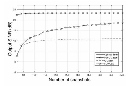
**Figure 8.** Output SINR versus snapshot number with SNR = SIR = 15 dB and  $1^{\circ}$  error.
