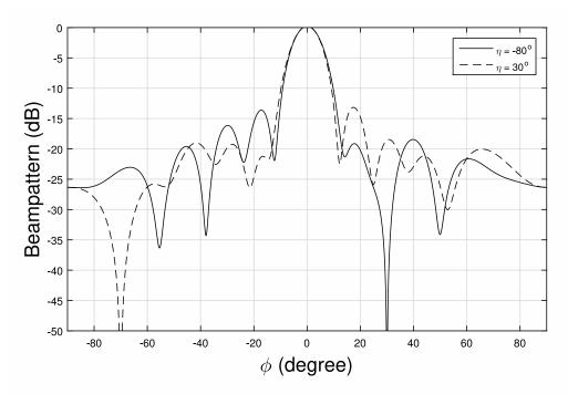
**Figure 3.** The resultant beam pattern for (1)  $\theta = 90^{\circ}$ ,  $\gamma = 60^{\circ}$ ,  $\eta = -80^{\circ}$ ; (2)  $\theta = 90^{\circ}$ ,  $\gamma = 60^{\circ}$ ,  $\eta = 30^{\circ}$ .
