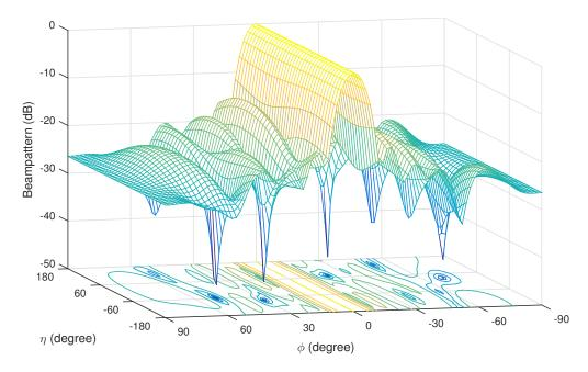
**Figure 2.** Beam pattern obtained from the full Q-Capon beamformer with  $\theta = 90^{\circ}$  and  $\gamma = 60^{\circ}$ .
