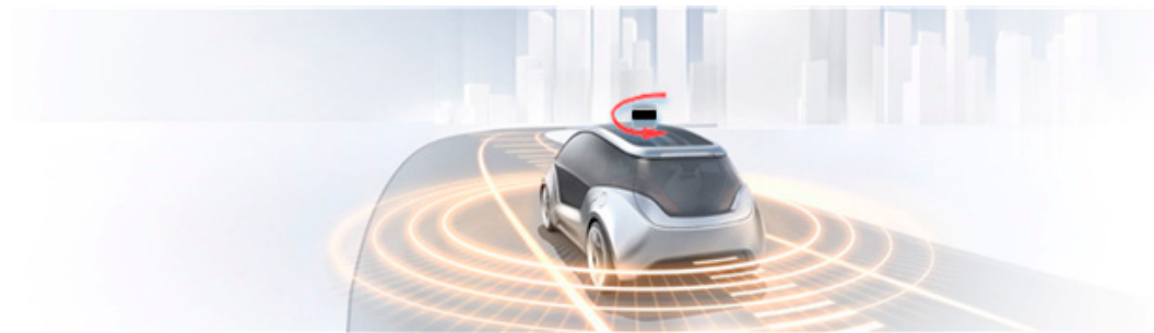
Figure 2. Example of a LiDAR sensor capable of 360° viewing angle working in constant rotation.
