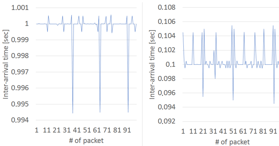
Figure 23. Jitter results ( left ): 1000 Byte packets, 1000 ms sending period, ( right ): 1000 Byte packets, 100 ms sending period with 50% background traffic.
