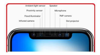
**Figure 32.** The iPhone X's notch is basically a Kinect.
