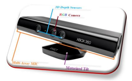
Figure 29. Microsoft Kinect Sensor.
