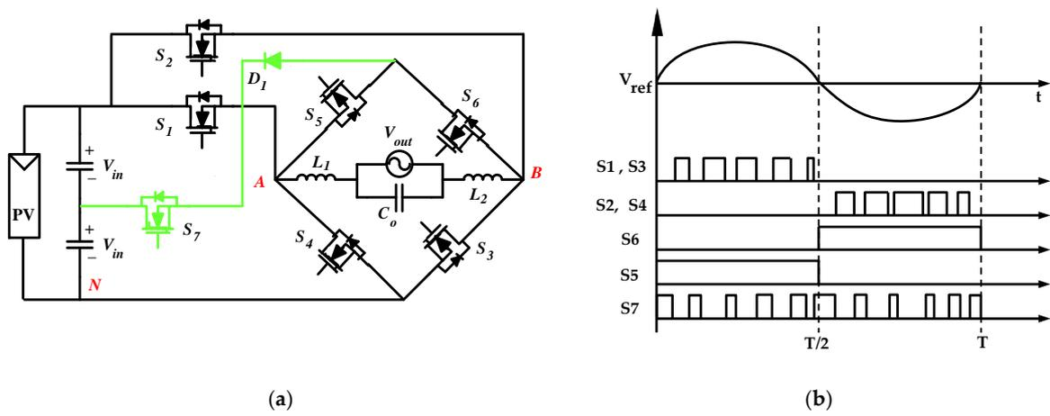
Figure 4. (a) The proposed topology, (b) Switching pattern.
