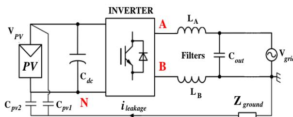
Figure 2. Equivalent circuit of a PV transformerless inverter.
