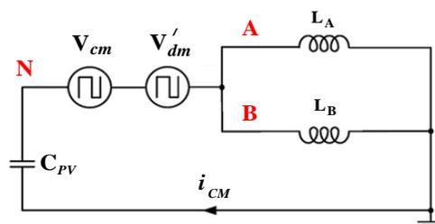
Figure 3. Common mode equivalent circuit.
