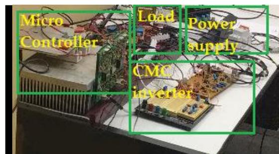
Figure 9. Laboratory setup of proposed H7-type inverter.
