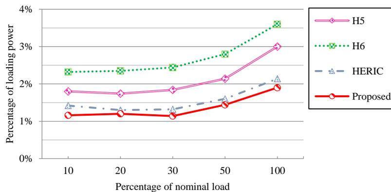
Figure 13. Total power loss through energy transmission.
