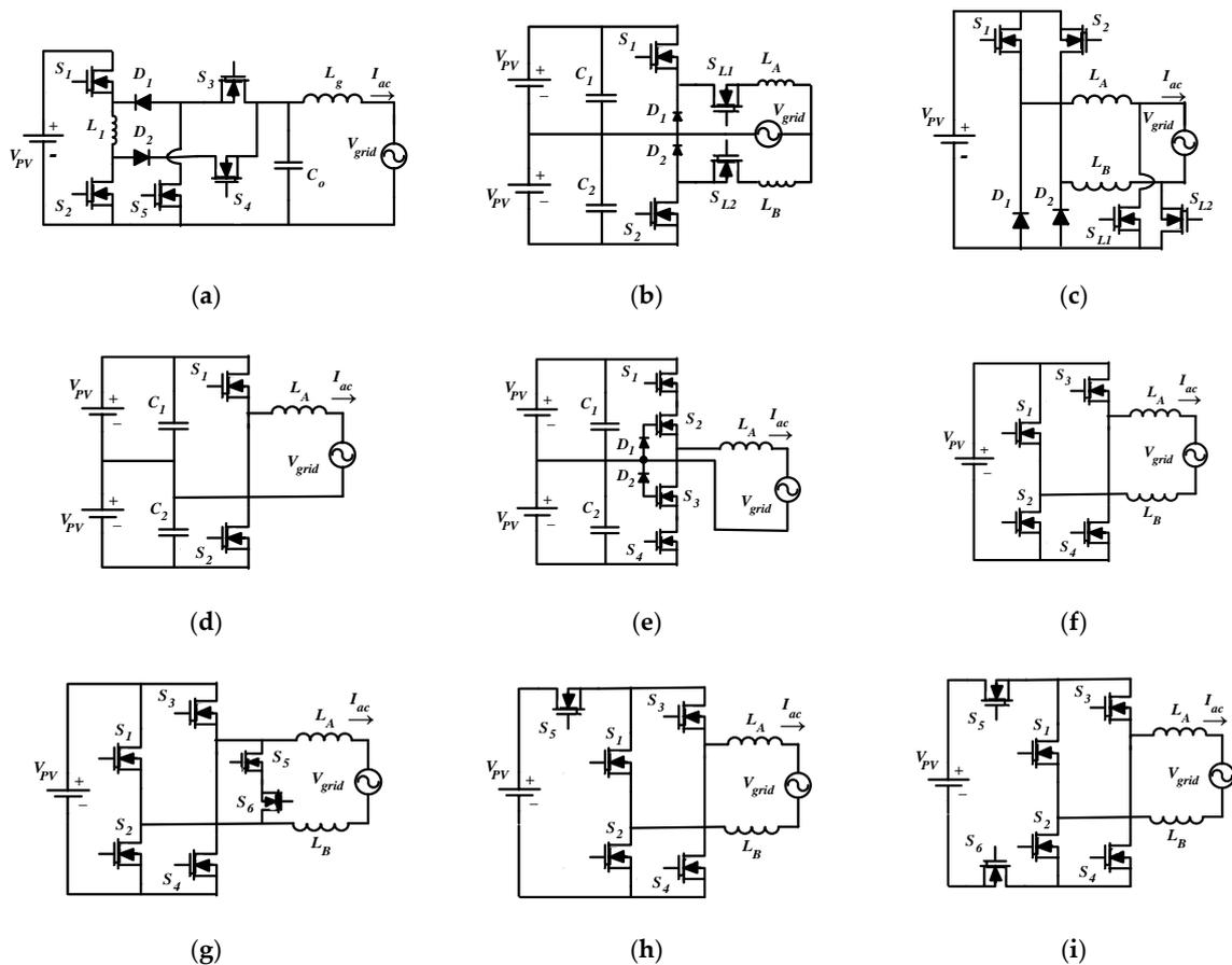
**Figure 1.** The main configurations of transformerless photovoltaic (PV) inverters in the literature. (a) Karschny [8], (b) series buck [9], (c) parallel buck [10], (d) half bridge [11], (e) neutral point clamped (NPC) [12], (f) full bridge [13], (g) highly efficient and reliable inverter (HERIC) [14], (h) H5 [15], (i) H6 [16].
