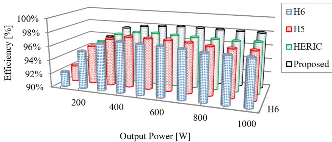
Figure 12. Efficiency evaluation in terms of output power.
