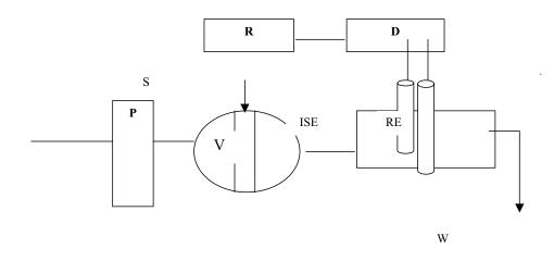
**Figure 2.** Single-stream FIA manifold for bromhexine hydrochloride determination; S, sample; P. peristaltic pump; V, injection valve; ISE, Brom-electrode; RE, reference electrode; D, detector. R, recorder; W, waste.
