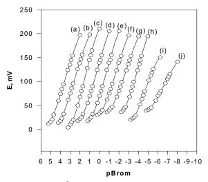
Fig. 1. Calibration graphs at 25<sup>o</sup>C for Brom-PT graphite coated electrode for 1h (a), 6h (b) and 24h (c), 3 (d), 6 (e), 9 (f), 12 (g), 14 (h), 15 (i) and 16 days (j).
