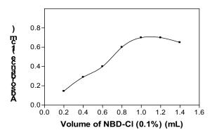
Fig. 3. Effect of volume of NBD-CI (0.1%) on the absorbance value of the reaction product of isoxuprine HCI (16 mg mL<sup>-1</sup>) at pH 7.8.
