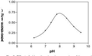
Fig. 2. Effect of pH on the absorbance value of the reaction product of isoxuprine HCI (16 μg mL<sup>-1</sup>) with NBD-CI
