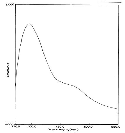
Fig. 1. Absorption spectrum of the reaction product of isoxsuprine HCl (20  $\mu$ g mL <sup>-1</sup>) with NBD-Cl at pH 7.8.
