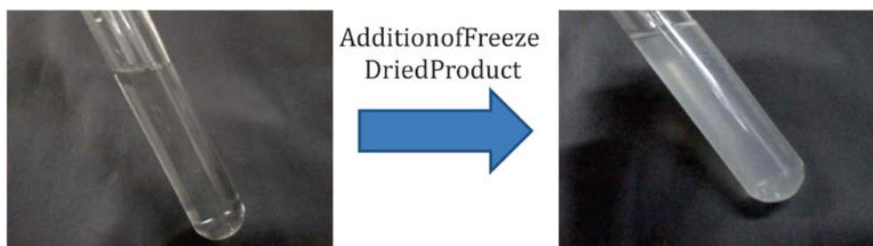
**Fig. 5.** Re-dispersibility of freeze-dried nanoparticles
