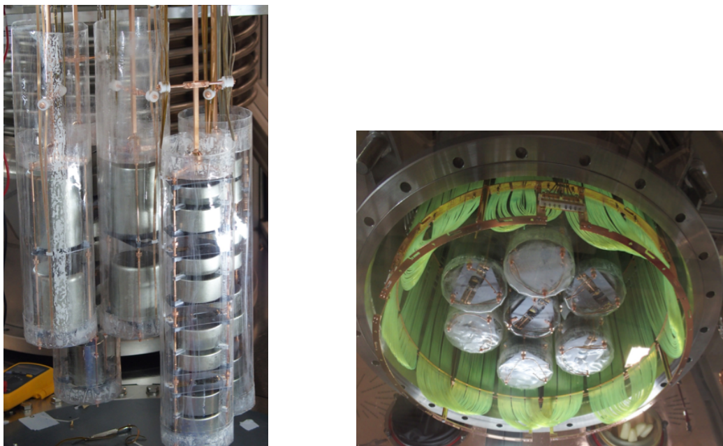
Figure 2. The Phase II Ge array with the individual Ge detector strings inserted in TPB coated nylon mini-shrouds (left) and the Fiber Shroud surrounding the detector strings once lifted up in the lock (right).
